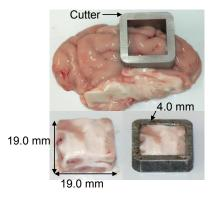
Fig. 2 – Square brain specimen  $(19.0 \pm 0.1 \times 19.0 \pm 0.1 \text{ mm})$  and  $4.0\pm0.1$  mm thick excised from medial to lateral direction. The prepared specimen is placed on a lower platen applied with a thin layer of surgical glue.
