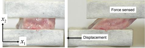
Fig. 4. The brain specimen attached between the platens using thin layer of surgical glue indicating tissue deformation before and after the completion of simple shear test.
