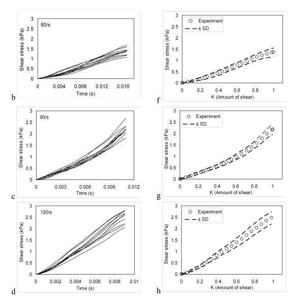
Fig. 5. Experimental shear stress profiles at each strain rate (left) and corresponding average stress and standard deviations (SD) shown on the right side.
