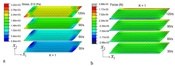
Fig. 9. Simple shear deformation using Ogden parameters (a) shear stress (Pa) contours (b) force (N) contours
