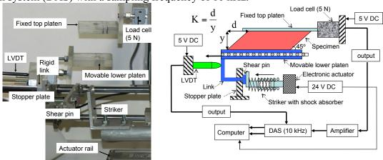
Fig. 1. (a) Major components of high rate shear device (HRSD), (b) Schematic diagram of complete test setup. K = 1 for maximum amount of shear
