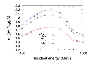
FIG. 6: Ratio of total reaction cross sections of  $^{12}$ C,  $^{16}$ O, and  $^{40}$ Ca for antiproton and proton scattering as a function of the incident energy.
