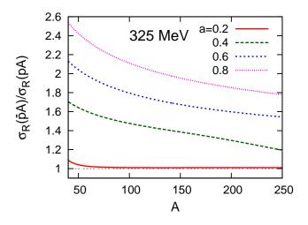
FIG. 7: Ratio of total reaction cross sections for antiproton and proton scattering at 325 MeV calculated using the 2pF density distributions with various diffuseness parameters as a function of the mass number A. See text for details.
