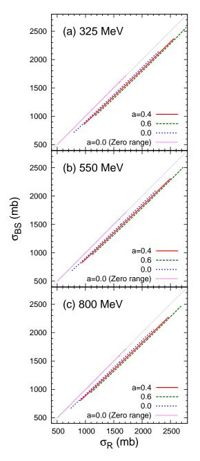
FIG. 9: Correlation plot of  $\sigma_{BS}$  versus  $\sigma_R$  at (a) 325, (b) 550, and (c) 800 MeV for the antiproton scattering. Thin lines in gray denote a y = x line for a guide of eyes.
