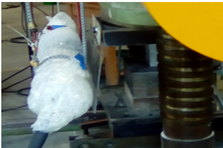
Figure 5: The mechanical press, the granite block inside its jaws and the detector, suspended and wrapped in a white protective plastics. The ^3\text{He} detection system was recalibrated against thermal neutrons with this protection in place.
