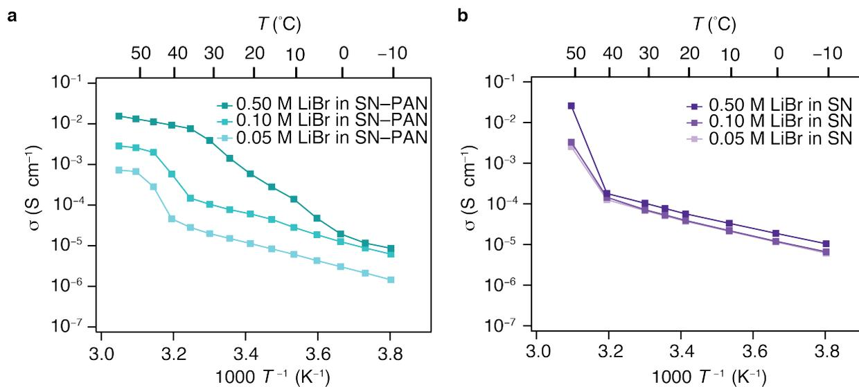
**Figure S4** (A) Temperature-dependent ionic conductivity of SN-PAN composite doped with  $[\text{LiBr}] = 0.05 \text{ M}$ ,  $0.10 \text{ M}$ , and  $0.50 \text{ M}$  (light cyan to dark cyan). (B) Temperature-dependent ionic conductivity of SN doped with  $[\text{LiBr}] = 0.05 \text{ M}$ ,  $0.10 \text{ M}$ , and  $0.50 \text{ M}$  (light purple to dark purple).
