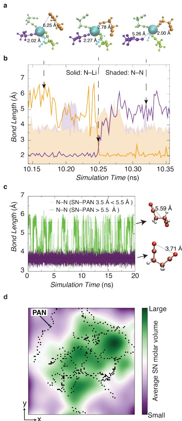
**Figure 3**  $\text{Li}^+$  and SN displacement dynamics within the SIC (A–B) The simulated bond length between the  $\text{Li}^+$  and SN within the first and second solvation shell (solid lines), as well as intra N–N distances for different SN molecules (shaded zone). The solvation shell of  $\text{Li}^+$  at different simulation times shows  $\text{Li}^+$  hopping between adjacent solvation sites assisted by the *trans* to
