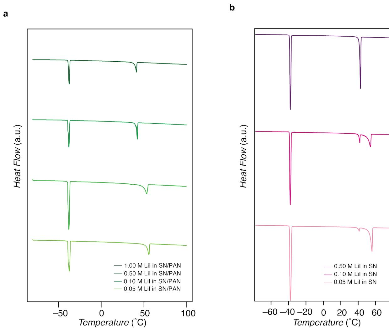
**Figure S8** (A) Differential scanning calorimetry (DSC) SN-PAN composites doped with [LiI] = 0.05 M, 0.10 M, 0.50 M, and 1.00 M (light green to dark green). (B) DSC of SN doped with [LiI] = 0.05 M, 0.10 M, and 0.50 M (light purple to dark purple).
