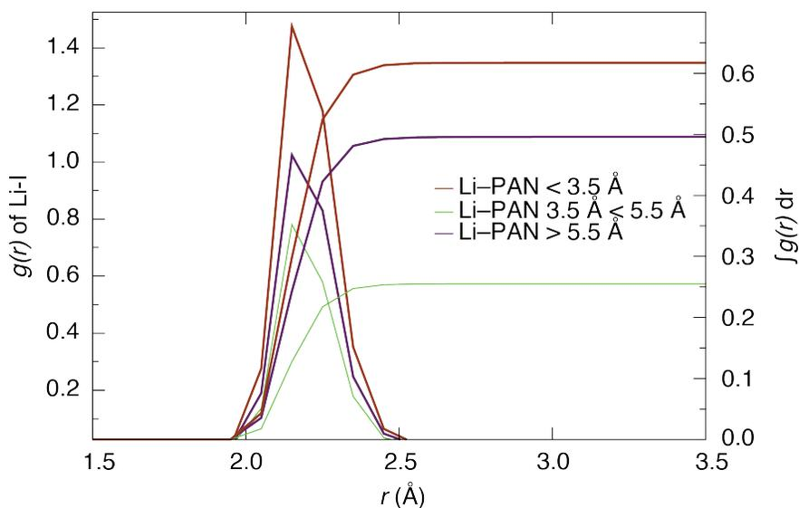
**Figure S6** Radial distribution function,  $g(r)$ , of  $\text{Li}^+$  concentration with respect to the distance from  $\text{I}^-$  within three domains in SIC—within 3.5 Å (brown zone), between 3.5 Å and 5.5 Å (green zone), and more than 5.5 Å (purple zone) from the PAN backbone.
