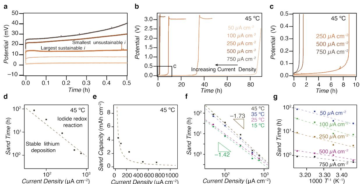
**Figure 6 Sand Analysis of the SIC composite.** (A) Time-dependent potential behavior of 150  $\mu\text{m}$  thick 1.00 M LiI-doped SN–PAN composite in response to applied current densities ( $50$  to  $750 \mu\text{A cm}^{-2}$ , light brown to dark down) for first 30 min at  $45 \text{ }^\circ\text{C}$ . The largest sustainable current
