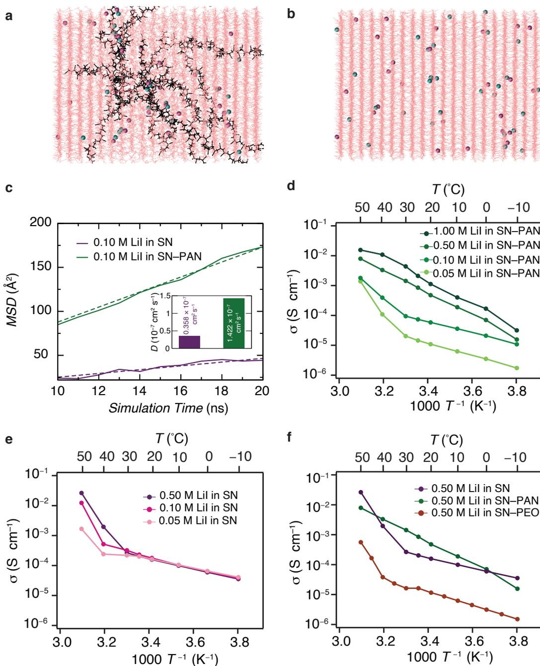
**Figure 1: Lithium transport through SIC composites.** (A) Simulated structure of a LiI-doped SN-PAN plastic crystal-polymer composite, showing SN molecules (light pink), 13 linear PAN chains (black), 0.10 M of  $\text{Li}^+$  (cyan) and  $\text{I}^-$  (pink). (B) Simulated structure of LiI-doped SN plastic crystal SIC. (C) Simulated mean square displacement (*MSD*) of  $\text{Li}^+$  as a function of simulation time
