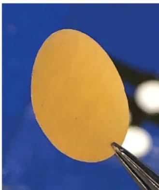
**Figure S1** Image of 150- $\mu\text{m}$  thick disk of 1.0 M LiI-doped SN-PAN composite solid-ion conductor (SIC).
