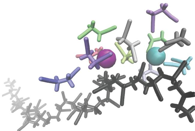
**Figure S2** Close up look at the PAN-SN interface inside the relaxed SIC simulation cell. The PAN (black), and the SN (different colored for clarity) in the vicinity of the  $\text{Li}^+$  (cyan) and  $\text{I}^-$  (purple). The longer segments pointing out of PAN backbone and on SN are the nitrile group, where the shorter ones are hydrogen.
