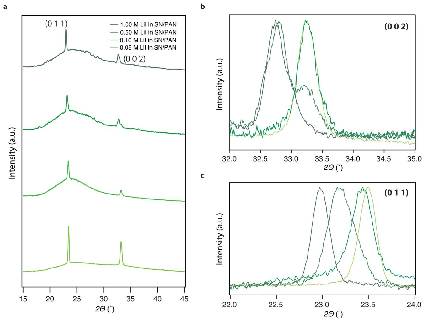
**Figure S5 (A-C)** X-Ray diffraction (XRD) patterns of SN-PAN composites doped with [Li] = 0.05 M, 0.10 M, 0.50 M, and 1.00 M (light green to dark green).
