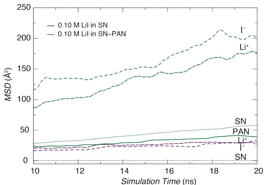
**Figure S7** The simulated mean square displacement ( $MSD$ ) of  $\text{Li}^+$ , SN molecules and  $\text{I}^-$  as a function of simulation time within 0.10 M LiI-doped SN-PAN composite SIC (green) and 0.10 M LiI-doped SN SIC (purple). It is evident from the  $MSD$  that translation motion of SN molecules is negligible in comparison to  $\text{Li}^+$  and  $\text{I}^-$  ions within the SIC.
