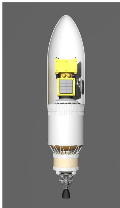
Figure 3 The Assembled Kinetic Impactor within the Long March 5 fairing
