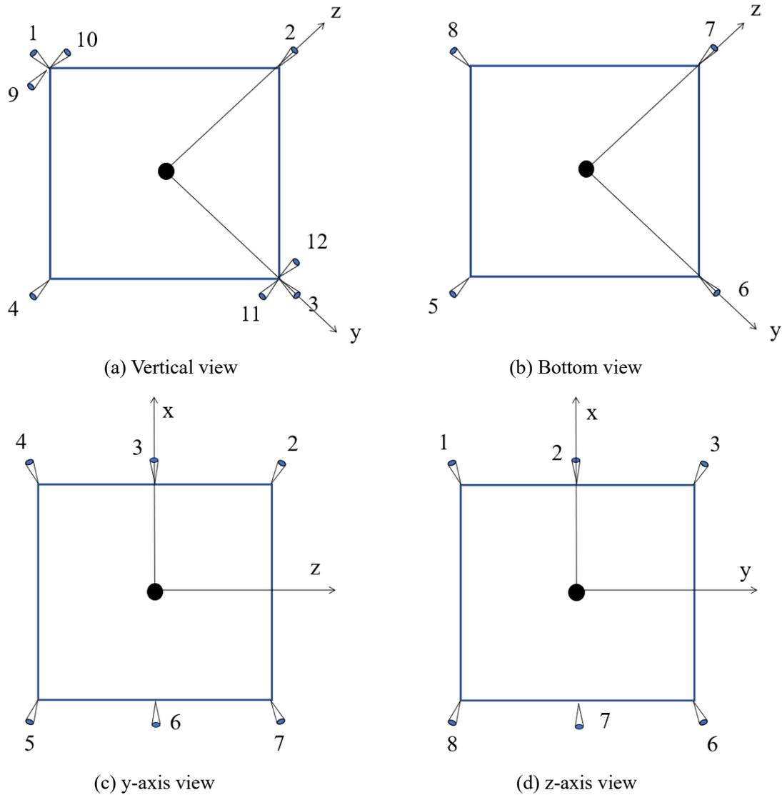
Figure 7 Thruster distribution in different views
