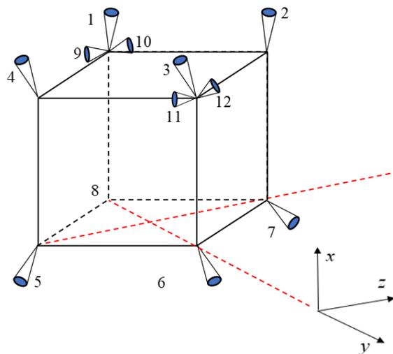
Figure 6 The schematic diagram of the thruster distribution (3-dimensional)
