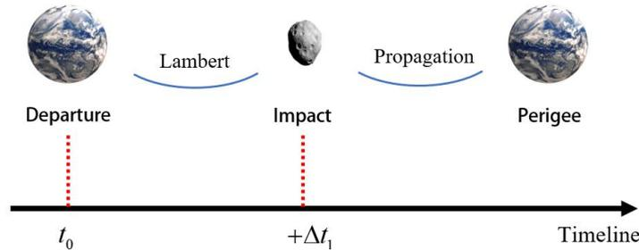
Figure 9 AKI transfer model. The AKI is launched from Earth at  $t_0$ , impact the asteroid after  $\Delta t_i$  days. By solving the Lambert problem, the hyperbolic excessive velocity  $\mathbf{v}_\infty$  at Earth's SOI and the impact velocity  $\mathbf{v}_{AKI}$  can be calculated. The  $\mathbf{v}_\infty$  can be provided by launch vehicle, and the corresponding spacecraft mass of the AKI can be calculated by launch capability.
