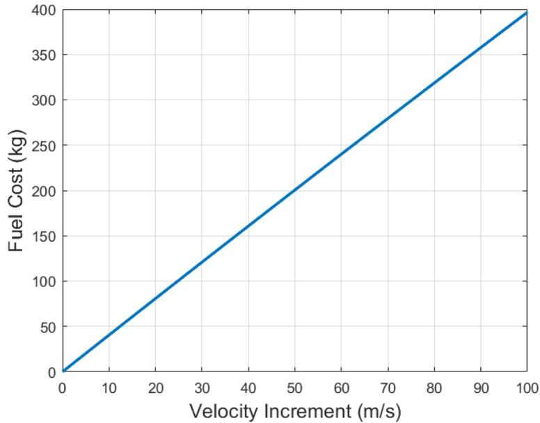
Figure 4 Fuel cost corresponding to the velocity increment of Assembled Kinetic Impactor
