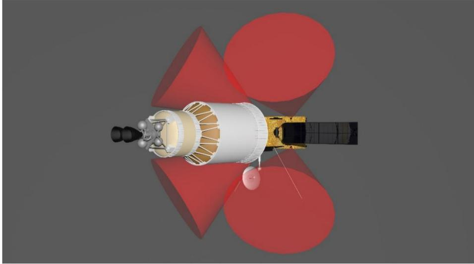
Figure 8 Analysis diagram of the thruster plumes
