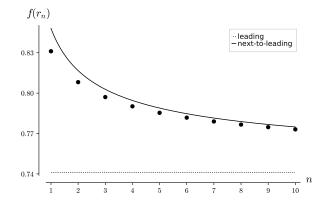
FIG. 2. The values  $f(r_n)$  obtained from the numerical solution of the exact critical vortex equations (black dots), the asymptotic value  $f(r_n) = e^{w_0}$  (dotted line), and the next-to-leading approximation (solid line) as functions of the winding number n.
