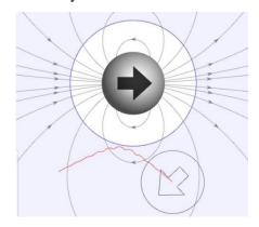
Fig. 5.22. 2D simulations of a spinning dipole body scattering from a static field using MagPhyx application. While the static field is produced by the central point dipole, rotating dipole body is shown by the other circle. The embedded arrows show the instantaneous direction of the dipole moment. Red traces show the travelled path of the spinning free body.
