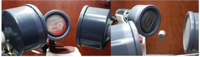
Fig. 5.33. A cylindrical magnet (the small object at the center of Fig. 5.34. Similar experiment of the left picture but the frame) is floating in air at the center of the equilateral triangular formation of large rotating magnet assemblies right has opposite rotation direction of the units at providing only AC fields (a cyclic field without static component). left.
