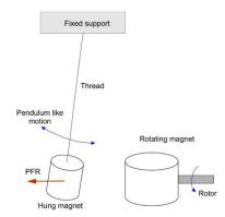
Fig. 5.24. Pendulum like configuration where a dipole magnet attached to a thread experiences PFR from another dipole magnet rotating on an axis orthogonal to dipole axis. The orientation and fixture point of the hung magnet is not important. Rotor velocity can be chosen in the 5000 - 15000 RPM range for a pendulum magnet of  $\emptyset 10 \times 10$  mm in size.
