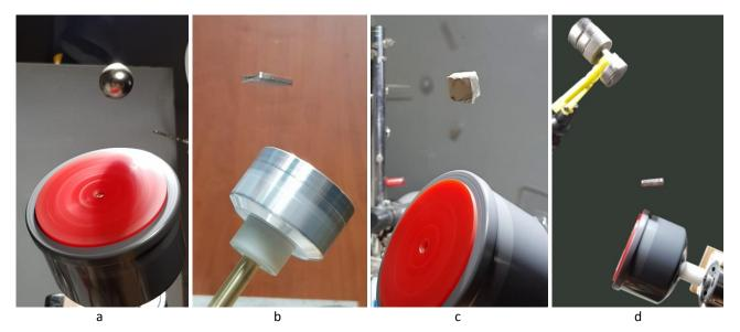
Fig. 5.18. Trapping configurations where various shaped floators are kept above rotators by the help of overhead magnets (shown on (d)) and the gravity in configurations where the rotator axis is not vertical. Rotators magnetic configurations do not generate static magnetic components and these can be seen in Fig. 5.35(g, h). In the configuration (d), overhead magnet position and orientation is hard to predict. Note: Background of this picture is erased for clarity.
