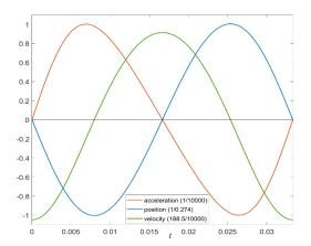
Fig. 5.9. Normalized plot of azimuthal position, angular velocity and acceleration of the body over one cycle of rotating field derived from data of numerical solution 1 from Table 5.4.
