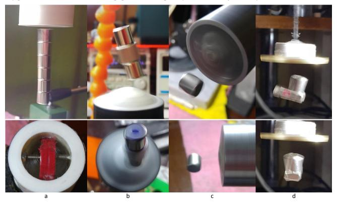
Fig. 5.21. Miscellaneous configurations where magnets held in air by interaction of a rotating magnets. (a) A stack of six  $\emptyset 10 \times 10$  mm magnets is trapped under a rotator assembly with a gap less than 4 mm. Here, the repulsive action is mostly
