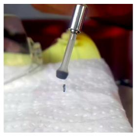
Fig. 1.1. A scaled-down MBS realization where a tiny fragment of a NdFeB magnet weighing about 5 mg is levitated at the tip of rotator assembly consisting of an irregular magnet fragment of  $\sim$ 3 mm in size coupled to a micro motor having dimensions  $\emptyset$ 4×10 mm running at 105000 RPM (11000 rad/s).
