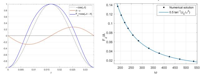
Fig. 5.15. (L) Plot of floator azimuthal motion  $\theta(t)$  and the *z* component of the force  $F_z(t)$  it receives for the configuration 1 at table 5.1. Red curve corresponds to angle  $\theta$  which varies between  $\pi \pm 0.275$ . The force  $F_z$  marked by the blue curve
