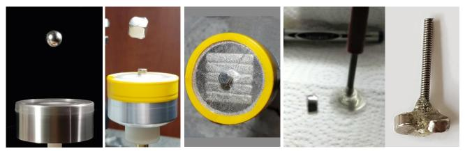
Fig. 5.29. A spherical dipole magnet Ø15 mm is levitating over a large rotating dipole magnet assembly by the help of an overhang magnet and gravity. In this configuration, magnetic forces are upward and are balanced by the weight of the floating magnet.
