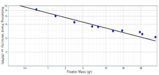
Fig. 5.26. Minimum frequency required for stability for levitating bodies obtained by tests using the same rotator configuration and using floators of different masses *m* but having similar geometries. This relation is reflected by the function  $\omega = a m^b$  by curve fitting method where the exponent b=-0.326. This shows a possible relation between  $\omega$  and body mass by its inverse cube root (b=-0.333).
