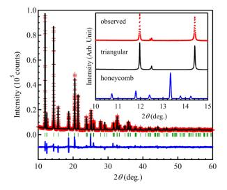
Fig. 1. Powder synchrotron X-ray diffraction patterns of  $Os_xCl_3$  at room temperature. The red crosses and solid black lines represent the observed data and Rietveld fit, respectively. The difference between them is indicated by the bottom blue line and the expected peak positions are shown as vertical green marks. The inset expands the low-angle region of the observed profile (top), which is compared with simulated profiles for the triangular (middle) and honeycomb structures (bottom).
