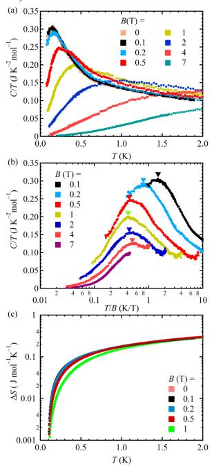
Fig. 6. (a) Temperature dependence of heat capacity divided by temperature under magnetic fields at T = 0.08-2 K, measured using a dilution refrigerator. (b) C/T plotted as a function of T/B. The triangles mark the top of the peaks. (c) Variations in entropy from 0.1 K to 2 K, obtained from the C/T data.
