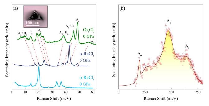
Fig. 7. (a) Raman spectra of  $Os_xCl_3$  at T = 300 K and ambient pressure. Those of  $\alpha$ -RuCl<sub>3</sub> at 0 GPa and 5 GPa (adapted from Ref. 44) are shown for comparison. An optical microscope image of the  $Os_xCl_3$  single crystal used for measurements is shown in the inset. (b) Raman spectrum of  $Os_xCl_3$  in an extended energy range up to 750 meV. The curve is a fit to the data.
