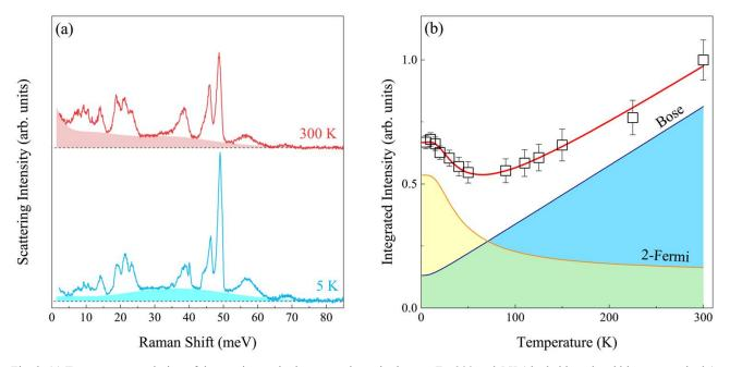
Fig. 8. (a) Temperature evolution of the continuum in the magnetic excitations at T = 300 and 5 K (shaded in red and blue, respectively). (b) Temperature dependence of the integrated intensity of the magnetic continuum (open squares). The intensity is fitted to a sum of bosonic (blue) and two-fermionic (yellow) excitations.
