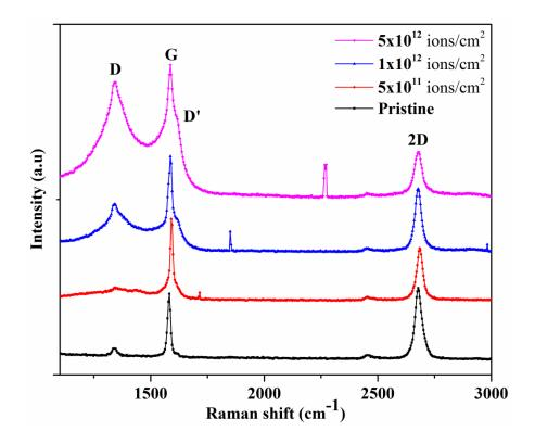
Fig. 2. Raman spectra of pristine and Si<sup>+5</sup> ion irradiated graphene.
