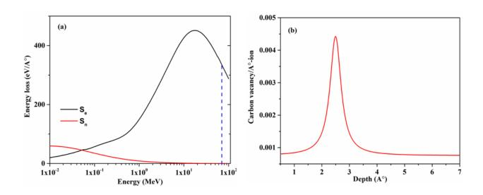
Fig. 9. (a) Electronic energy loss and nuclear energy loss of  $Si^{+5}$  ions in graphene. (b) Carbon vacancies in graphene.
