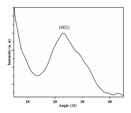
Fig. 1. XRD plot of pristine graphene. The peak at  $\sim 24^{\circ}$  corresponds to the (002) plane.
