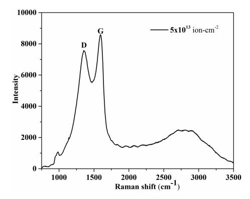
**Fig. 5.** Raman spectrum of Si<sup>+5</sup> beam irradiated graphene with fluence  $5 \times 10^{13}$  ions-cm<sup>-2</sup>; complete transformation of graphene into amorphous carbon is visible.
