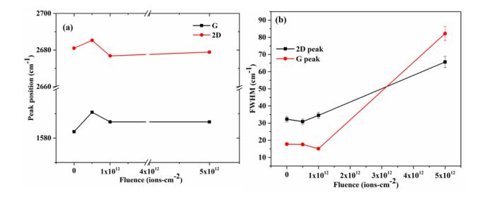
**Fig. 3.** (a) 2D and G Raman peak position vs. fluence in pristine and irradiated graphene. (b) FWHM of 2D and G peaks vs. fluence.
