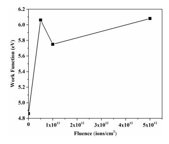
Fig. 8. WF evolution of graphene under ion irradiation.
