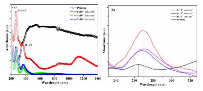
Fig. 6. (a) Absorbance spectra of pristine and irradiated graphene. (b) Zoomed view of the peak at ~265 nm.
