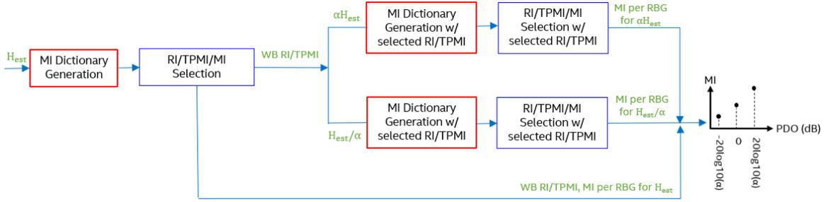
Fig. 2. An example of the block diagram for generating WB RI, WB TPMI, and MI per RBG as a function of PDO.
