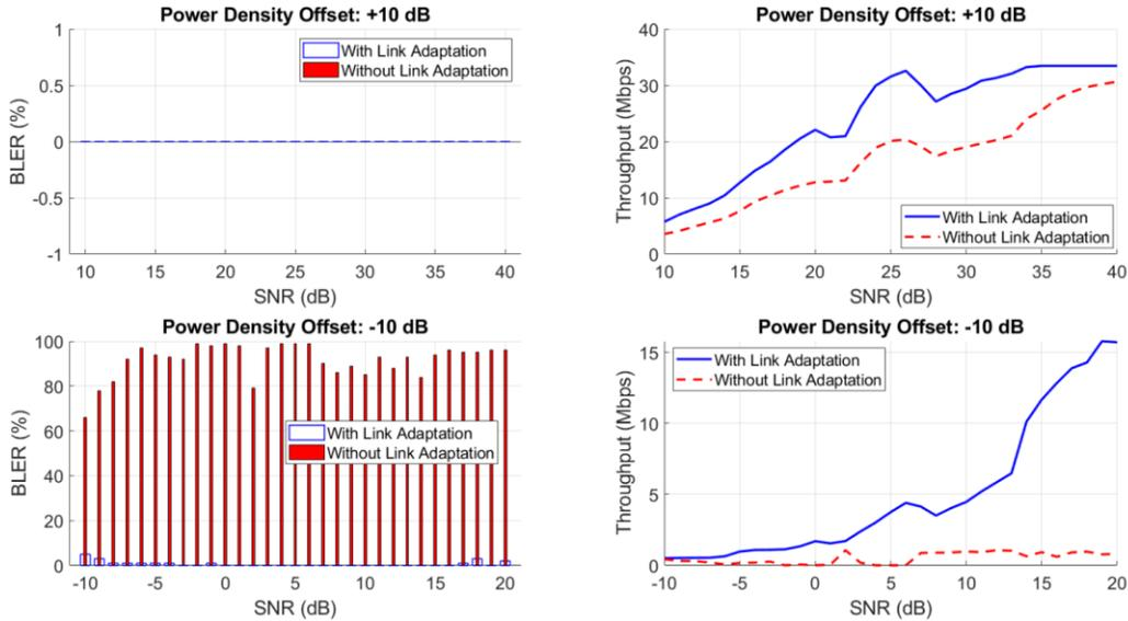
Fig. 4. Comparison of BLERs and throughput between without and with link adaptation cases for PDOs of +10 dB (top) and -10 dB (bottom). The channel is 4x4 EPA5, and the SRS transmission comb is 4.
