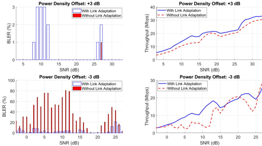
Fig. 3. Comparison of BLERs and throughput between without and with link adaptation cases for PDOs of +3 dB (top) and -3 dB (bottom). The channel is 4x4 EPA5, and the SRS transmission comb is 4.
