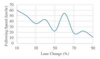
Fig. 5. Change in observed passenger car lane change behavior when following heavy vehicles at various speeds.
