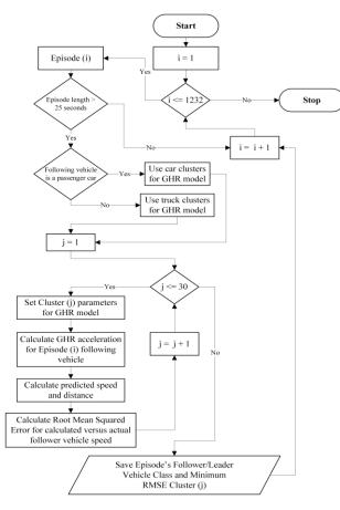
Fig. 3. Flowchart showing the data flow of the MATLAB code used for GHR regression.
