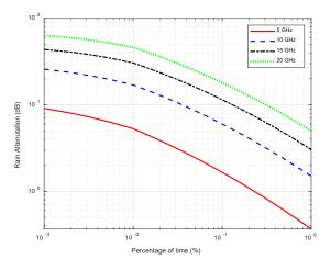
Fig. 5. Specific attenuation losses due to rain versus the percentage of rain time for different navigation signal frequencies
