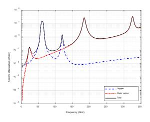
Fig. 4. Specific attenuation losses due to atmospheric gases versus the navigation signal frequency
