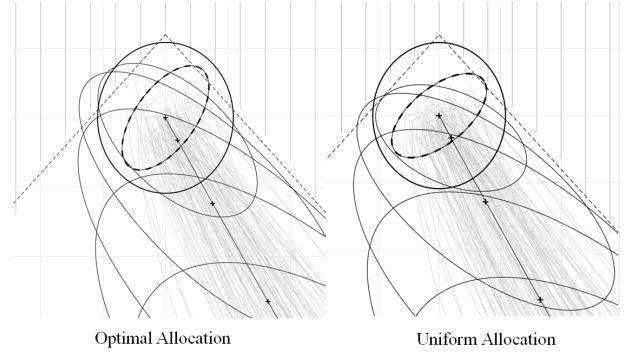
Fig. 4: Comparison of terminal covariance steering using a uniform and the optimal risk allocation.
