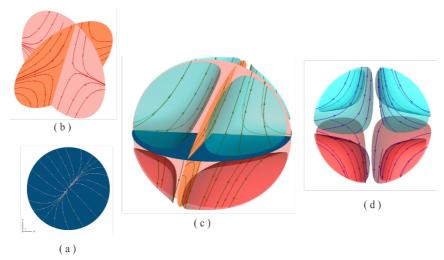
Fig. 4. Local streamline pattern of velocity gradient with three real eigenvalues: (a) the foci plane of streamlines normal to  $m_3$ , namely the eigenvectors related to the eigenvalue with the maximal module, (b) two saddle planes of streamlines normal to the eigenvectors related to two eigenvalues with smaller modules, (c) local streamline pattern divided by three base planes, (d) local streamline pattern removing three base planes.
