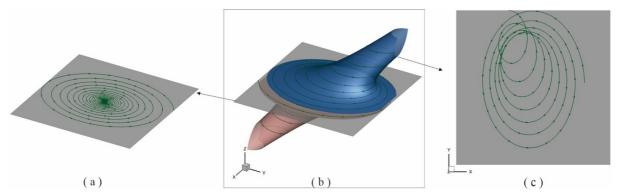
**Fig. 3**. Local streamline pattern of velocity gradient with a unique real eigenvalue: (a) the base plane and the streamline on it, (b) local streamline pattern, (c) the projection of an above streamline on the base plane.
