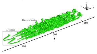
Fig. 7. The DNS data of the flat boundary flow with Mach number of 0.5, shown with criterion  $\Omega = 0.52$ .
