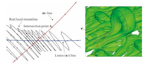
Fig. 9. A real local streamline and its direction features observed following a fluid particle in the leg of a typical vortex.
