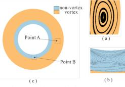
**Fig. 5**. The property of Liutex in the Taylor-Couette flow: (a) local streamlines for the velocity gradient at point A in vortex region, (b) local streamlines for the velocity gradient at point B in non-vortex region, (c) division of vortex and non-vortex regions.
