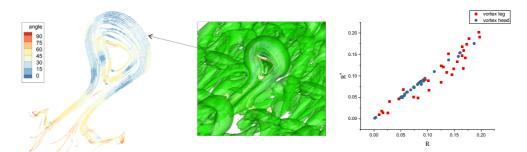
Fig. 8. The distribution of included angle between  $m_3$  and  $n_3$  on a typical hairpin-vortex. In the left Liutex lines extracted from the middle field with typical vortices, the blue color in the head and junction shows the small included angle while the red color mainly in the leg shows the large included angle. The right is the correlation between R and R<sup>\*</sup> using 30 random samples from the leg and head, respectively.
