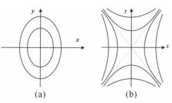
Fig. 2. Local streamline pattern of two-dimensional flows at point where the velocity gradient tensor has: (a) complex eigenvalues, (b) real eigenvalues.
