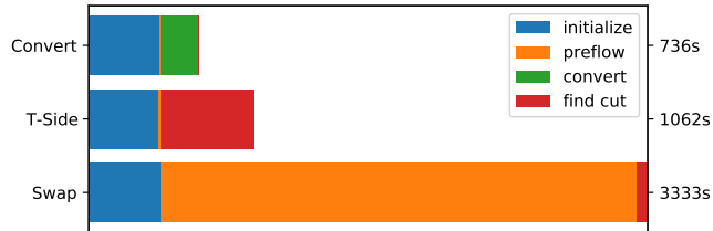
Figure 7: Distribution of spent time during Gusfield’s algorithm on the soc-slashdot instance with three approaches to use the Push-Relabel algorithm as a min-cut oracle. We split the measurements into initialization, preflow, conversion, and cut identification. The time overhead for measurement, logging, and the logic of Gusfield’s algorithm is included in the numbers on the right but excluded in the bars.
