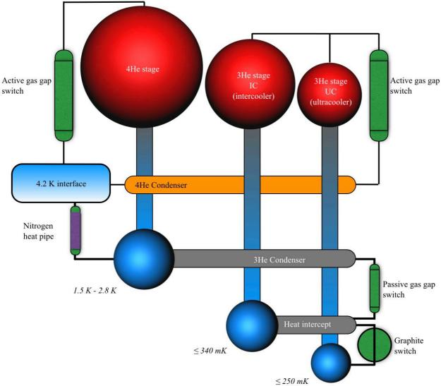
Figure 3. Schematic of the 3 stages cooler
