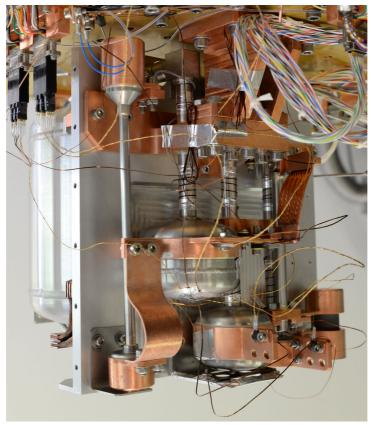
Figure 5. Cooler in the test cryostat
