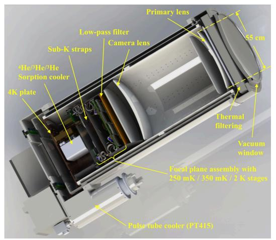
Figure 1. Schematic of the BICEP Array telescope
