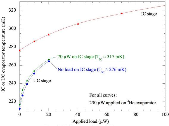
Figure 7. Cooling power of IC and UC stages
