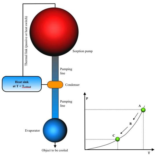
Figure 2. Principle of operation of a sorption cooler: [A] condensation, [B] cooldown and [C] low temperature
