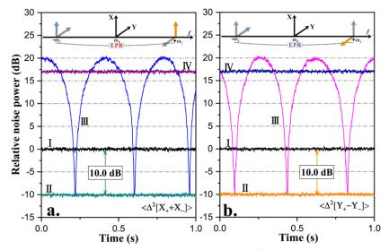
Fig. 3 Normalized correlation noise of amplitude-sum (a) and phase-difference (b) between the upper and lower sidebands  $\omega_0 \pm \omega_f$ . Trace I, shot noise limit; Trace II, correlation noise of  $<\Delta^2 [X_++X_-]>$  (a) and  $<\Delta^2 [Y_+-Y_-]>$  (b); Trace III, correlation noise variance with one of the BHD's phases of 0 (a) and  $\pi/2$  (b) while another BHD's phase is scanned linearly in time; Trace IV, noise spectrum with one of the BHD signal port is blocked.
