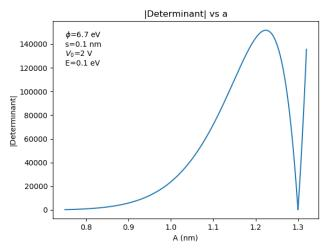
Fig. 6. Magnitude of the determinant as a function of the length of the tunneling junction where the work function is 6.7 eV, the applied potential is 2 V, the electron energy is 0.1 eV, and the pre-barrier length is 0.1 nm. The second resonance is at a = 1.300 nm.
