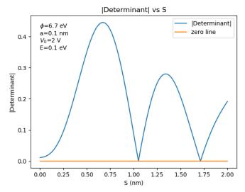
Fig. 8. Magnitude of the determinant as a function of the length of the pre-barrier region where the length of the tunneling junction is 0.1 nm. The work function is 6.7 eV, the potential is 2.0 V, and the electron energy is 0.1 eV,
