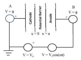
Fig. 1. Circuit model for the dynamic solution by Tien and Gordon [18].
