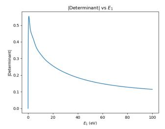
Fig. 10. Magnitude of the determinant as a function of the energy of the electrons where the length of the tunneling junction is 0.1 nm and the work function is 6.7 eV. The applied potential is 2 V and the pre-barrier length is 0.1 nm.
