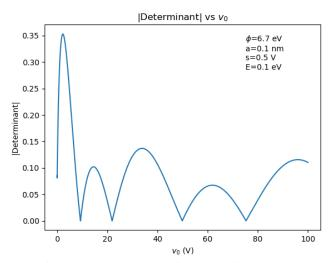
Fig. 9 shows the magnitude of the determinant as a function of the applied potential where the length of the tunneling junction is 0.1 nm, the work function is 6.7 eV and the electron energy is 0.1 eV. The length of the pre-barrier region is 0.5 nm and the first zero is at a potential of 9.30019 V.
