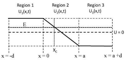
Fig. 11. Potential energy U for a model with quasistatic excitation of a tunneling junction shown at a time when  $E_x < 0$ .
