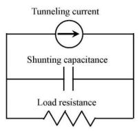
Fig. 12. Equivalent circuit measurements in laser-assisted scanning tunneling microscopy.
