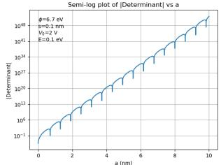
Fig. 5. Magnitude of the determinant as a function of the length of the tunneling junction where the work function is 6.7 eV, the applied potential is 2 V, the electron energy is 0.1 eV, and the pre-barrier length is 0.1 nm
