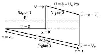
Fig. 4. Potential energy for a model of quantum tunneling in a static potential barrier.
