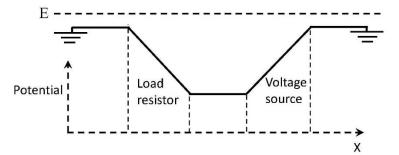
Fig. 2. Model showing a resistor, a voltage source, and lossless connectors.
