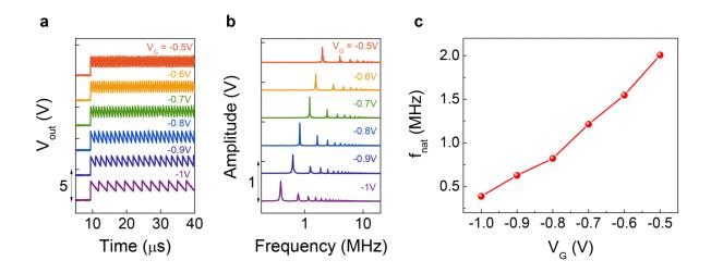
Fig. 3. Frequency-tunability of the 1OTS+1FET oscillator. a Output waveforms of the 1OTS+1FET oscillator for various  $V_{GS}$ . b Fast Fourier transform (FFT)-amplitude of the output waveforms. c Dependence of the natural frequency ( $f_{nat}$ ) on  $V_G$ , where  $f_{nat}$  is defined as the position of the primary peak in FFT.
