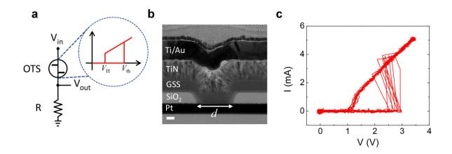
Fig. 1 Frequency-tunable nano-oscillator based on OTS device. a 10TS+1R structure as a basic oscillator device. The inset shows a schematic *I-V* curve of an OTS device. b A cross-sectional TEM image of an OTS device, where GSS means  $Ge_{37}Sn_{13}Se_{50}$  (scalebar=50 nm). c Characteristic *I-V* curve of an OTS device (ten repetitions).
