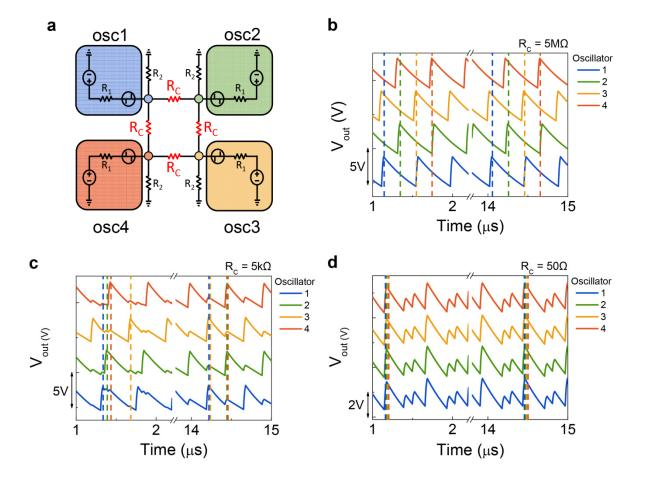
Fig. 5. Spice simulation of dynamics of a network composed of four coupled oscillators.
