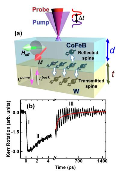
**Figure 2.** (a) Schematic of experimental geometry and (b) typical TR-MOKE data from  $Co_{20}Fe_{60}B_{20}(3 \text{ nm})/SiO_2(2 \text{ nm})$  heterostructure at an applied bias magnetic field of 2.30 kOe. The three important temporal regimes are indicated in the graph. The solid red line shows a biexponential fit to the decaying background of the time-resolved Kerr rotation data.
