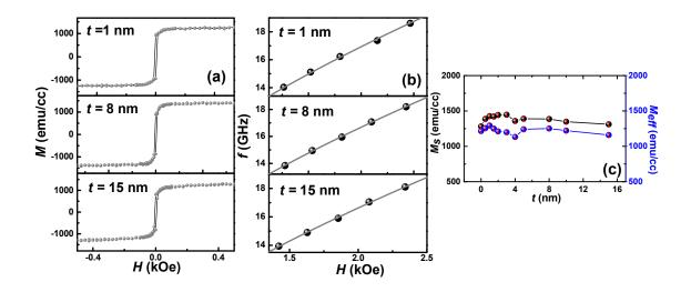
**Figure S3.** (a) VSM loops for W(*t*)/Co<sub>20</sub>Fe<sub>60</sub>B<sub>20</sub>(3 nm)/SiO<sub>2</sub>(2 nm). (b) Kittel fit (solid line) to experimental data (symbol) of precessional frequency vs. magnetic field for W(*t*)/Co<sub>20</sub>Fe<sub>60</sub>B<sub>20</sub>(3 nm)/SiO<sub>2</sub>(2 nm) samples. (c) Comparison of variation of  $M_s$  from VSM and  $M_{eff}$  from TR-MOKE as a function of W layer thickness.
