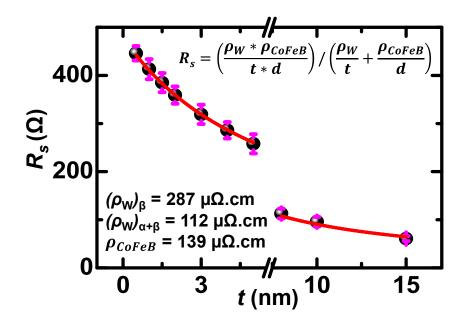
**Figure S1.** Variation of sheet resistance ( $R_s$ ) of the W (t)/ Co<sub>20</sub>Fe<sub>60</sub>B<sub>20</sub>(3 nm) film stack vs. W thickness t used for the determination of resistivity of the W and Co<sub>20</sub>Fe<sub>60</sub>B<sub>20</sub> layers.
