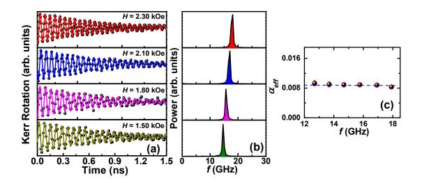
**Figure S6.** (a) Background subtracted time-resolved precessional oscillations at different bias magnetic fields for Sub/W(0.5 nm)/Co<sub>20</sub>Fe<sub>60</sub>B<sub>20</sub>(3 nm)/SiO<sub>2</sub>(2 nm) sample, where symbols represent the experimental data points and solid lines represent fits using equation (12) of the article. (b) The FFT power spectra of the time-resolved precessional oscillations showing the
