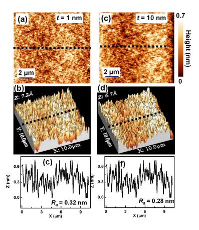
**Figure S2.** (a) The two-dimensional AFM image, (b) the three-dimensional AFM image, and (c) the line scan profile along the black dotted line for W(1 nm)/  $Co_{20}Fe_{60}B_{20}(3 nm)$  /SiO<sub>2</sub>(2 nm) sample. (d) The two-dimensional AFM image, (e) the three-dimensional AFM image, and (f) the line scan profile along the black dotted line for W(10 nm)/  $Co_{20}Fe_{60}B_{20}(3 nm)$  /SiO<sub>2</sub>(2 nm) sample.
