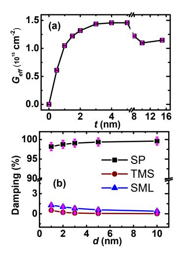
**Figure 5.** (a) Variation of effective spin-mixing conductance( $G_{eff}$ ) with W layer thickness *t* (symbol). The solid line is guide to the eye. (b) Contributions of SP, SML and TMS to the modulation of damping for different Co<sub>20</sub>Fe<sub>60</sub>B<sub>20</sub> layer thickness *d* (symbol). The solid line is guide to the eye.
