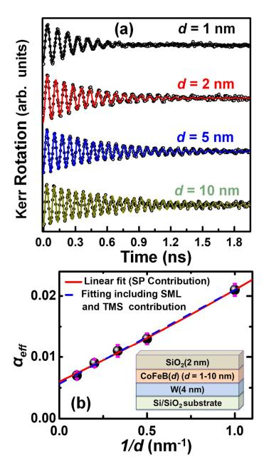
**Figure 4.** (a) Background subtracted time-resolved Kerr rotation data showing precessional oscillation for Sub/W (4 nm)/Co<sub>20</sub>Fe<sub>60</sub>B<sub>20</sub> (*d*)/SiO<sub>2</sub> (2 nm) as function of Co<sub>20</sub>Fe<sub>60</sub>B<sub>20</sub> thickness *d* at an applied bias magnetic field of 2.30 kOe. (b) Experimental result of variation of damping vs 1/d (symbol) fitted with theoretical models (solid and dashed lines).
