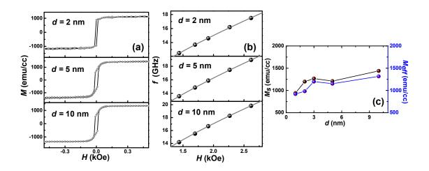
**Figure S4.** (a) VSM loops for W(4 nm)/  $Co_{20}Fe_{60}B_{20}(d)/SiO_2(2 nm)$ . (b) Kittel fit (solid line) to experimental data (symbol) of precessional frequency vs. magnetic field for W(4 nm)/  $Co_{20}Fe_{60}B_{20}(d)/SiO_2(2 nm)$  samples. (c) Comparison between variation of  $M_s$  from VSM and  $M_{eff}$  from TR-MOKE as a function of  $Co_{20}Fe_{60}B_{20}$  layer thickness.
