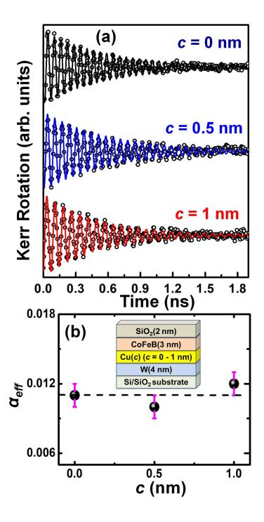
**Figure 6.** (a) Background subtracted time-resolved Kerr rotation data showing precessional oscillation for Sub/W(4 nm)/Cu(c)/Co<sub>20</sub>Fe<sub>60</sub>B<sub>20</sub>(3 nm)/SiO<sub>2</sub>(2 nm) as function of Cu layer thickness c at an applied bias magnetic field of 2.30 kOe. (b) Experimental result of variation of damping vs c. The dotted line is guide to the eye, showing very little dependence of damping on Cu layer thickness.
