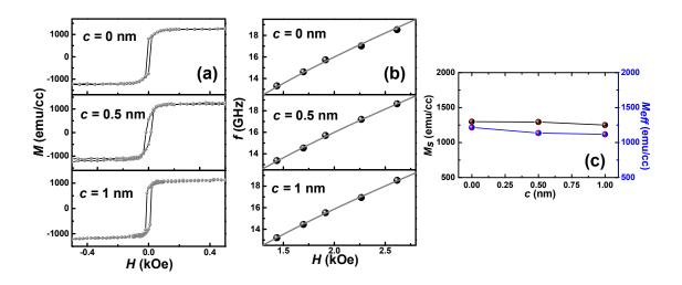
**Figure S5.** (a) VSM loops for W(4 nm)/Cu(*c*)/ Co<sub>20</sub>Fe<sub>60</sub>B<sub>20</sub>(3 nm)/SiO<sub>2</sub>(2 nm). (b) Kittel fit (solid line) to experimental data (symbol) of precessional frequency vs. magnetic field for W(4 nm)/ Cu(*c*)/ Co<sub>20</sub>Fe<sub>60</sub>B<sub>20</sub>(3 nm)/SiO<sub>2</sub>(2 nm) samples. (c) Comparison between variation of  $M_s$  from VSM and  $M_{eff}$  from TR-MOKE as a function of Cu layer thickness.
