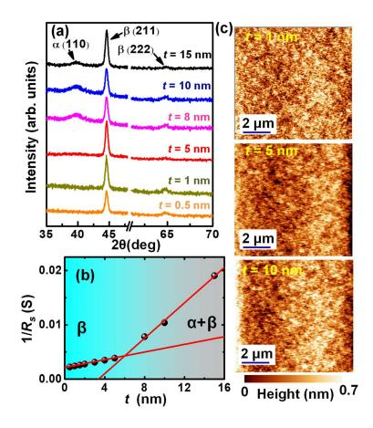
**Figure 1.** (a) X-ray diffraction patterns measured at 2° grazing angle incidence for different W thickness. (b) Variation of inverse sheet resistance with W thickness. (c) AFM images of the samples showing the surface topography.
