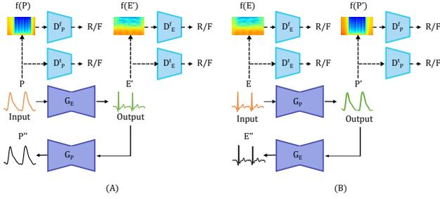
Figure 1: The architecture of the proposed CardioGAN is presented. The original ECG ( $E$ ) and PPG ( $P$ ) signals are shown in the color ‘orange’; the generated outputs ( $E'$  and  $P'$ ) are represented with the color ‘green’; and the reconstructed or cyclic outputs ( $E''$  and  $P''$ ) are marked with the color ‘black’ for better visibility. Moreover, connections to the generators are marked with solid lines, whereas, connections to the discriminators are marked with dashed lines.
