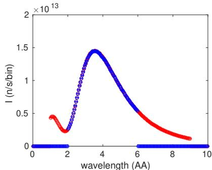
Figure 3: The simulation results obtained from shooting neutron rays from `Source_Maxwell_3()` into an `L_Mon()`, in effect showing the wavelength distribution of the source intensity. The Maxwellian source is run with two non-zero intensities, one corresponding to  $T = 300$  K, and one corresponding to  $T = 30$  K. The red points show the outcome of the source set with `Lmin=1` and `Lmax=9`; the blue points show the outcome where the two wavelength values are 2 and 6, respectively.
