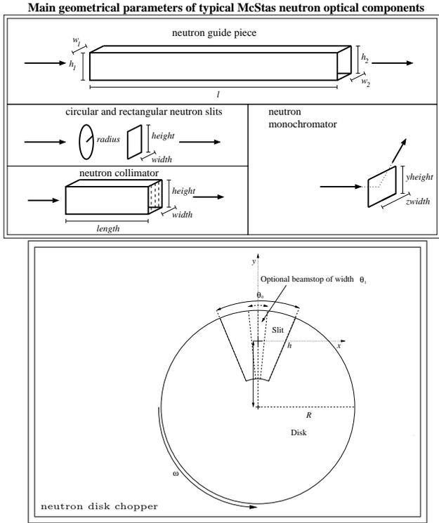
Figure 5: Geometries of the five described beam-optical elements with the standard naming of geometrical parameters shown.
