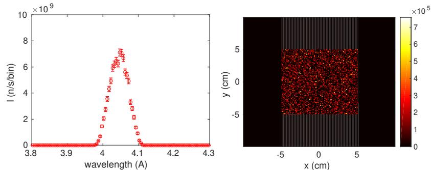
Figure 7: The simulation results obtained from the simple two-axis diffractometer in Fig. 6. (left) the wavelength distribution on the sample position as measured by `L_monitor()`. (right) The beam profile on the detector, measured by `PSD_monitor()`.
