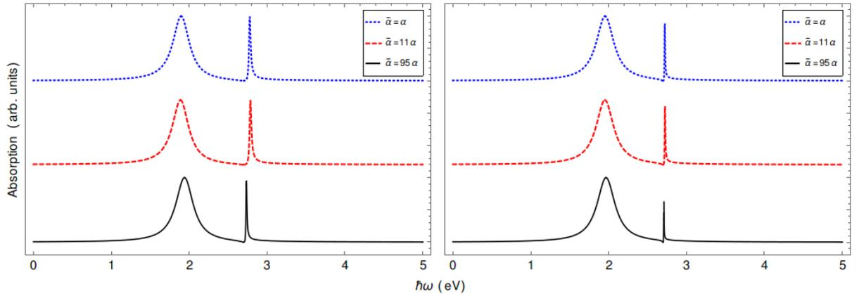
Fig. 4: Optical absorption spectrum of the TI-QD hybrid for longitudinal (left) and transverse (right) coupling for the rescaled topological magnetoelectric polarizabilities  $\tilde{\alpha} = \alpha$  (dotted blue line),  $\tilde{\alpha} = 11\alpha$  (dashed red line), and  $\tilde{\alpha} = 95\alpha$  (continuous black line). Here we fix  $\hbar\omega_\alpha = 2.7$  eV and  $r = 7$  nm.
