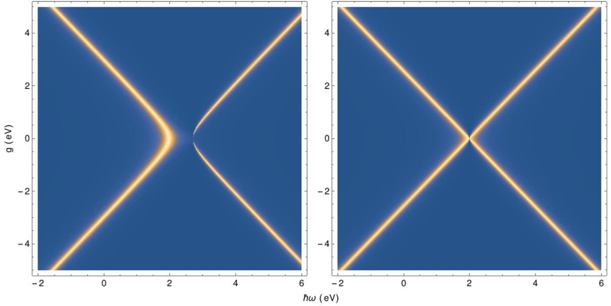
Fig. 2: Density plot of the optical absorption spectrum of the TI-QD hybrid as a function of the coupling strength ( $g$ ) and the energy  $\hbar\omega$  of the photonic field, for longitudinal (left) and transverse (right) coupling. The TI-QD Fano resonance achieve its maximum approach for the QD resonance energy  $\hbar\omega_\alpha = 2.0$  eV.
