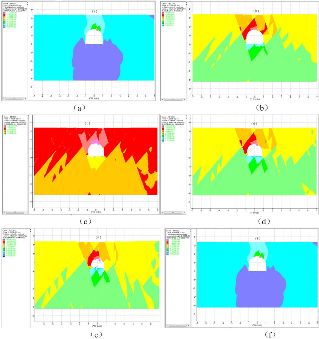
**Fig.4 Displacement cloud images of one to five explosions and tunnel under natural conditions**
