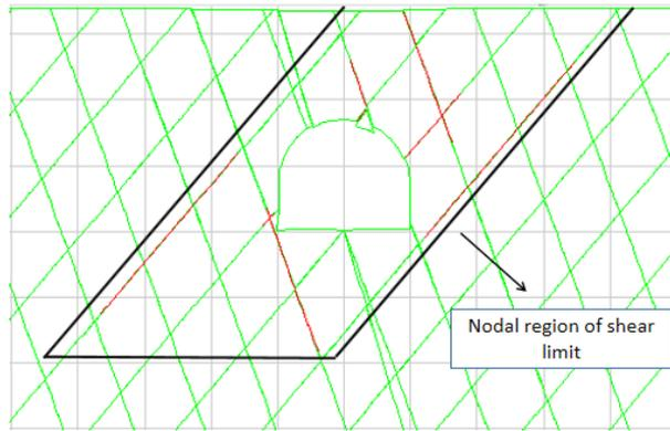
**Fig.5 Node graph of shear limit after the first blasting**
