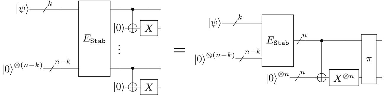
FIG. 1. Encodings of  $\mathcal{C}_{\text{Stab,KLM}}$  from the encoding  $E_{\text{Stab}}$  of  $\mathcal{C}_{\text{Stab}}$ . On the right side, CNOTs apply transversally to each pair of control and target qubits in the code blocks. The permutation  $\pi$  maps the  $j$ th qubit in the first block of  $n$  qubits to the  $(2j - 1)$ th qubit and the  $j$ th qubit in the second block of  $n$  qubits to the  $(2j)$ th qubit.
