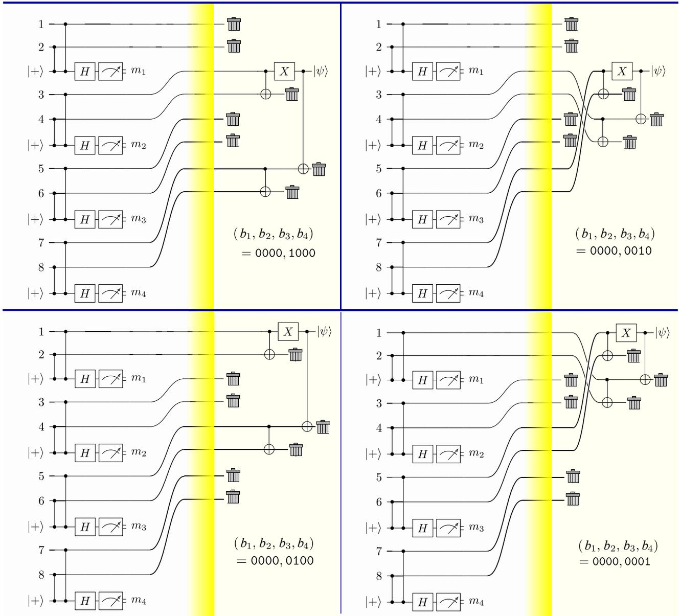
FIG. 4. Syndrome extraction and decoding of  $\mathcal{C}_{8\text{qubit}}$ . The syndrome vector is  $\mathbf{b} = (b_1, b_2, b_3, b_4) = (1 - (m_1, m_2, m_3, m_4))/2$ . If the Hamming weight of the syndrome vector is one, we can still correctly decode the logical qubit. For this, we discard four qubits and subsequently employ the same decoding circuit up to a permutation. If the Hamming weight of  $\mathbf{b}$  is 0, we can use any of the above decoding circuits.
