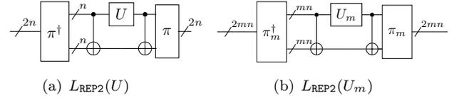
FIG. 2. Given single-qubit and multi-qubit logical operators of  $\mathcal{C}_{\text{Stab}}$  denoted by  $U$  and  $U_m$  respectively, we obtain corresponding logical operators for  $\mathcal{C}_{\text{Stab,REP2}}$  in (a) and (b) respectively. The permutation  $\pi_m$  maps the  $j$ th qubit in the first block of  $mn$  qubits to the  $(2j - 1)$ th qubit and the  $j$ th qubit in the second block of  $mn$  qubits to the  $(2j)$ th qubit.
