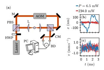
FIG. 1. (a) Schematic of the dual beam optical trap and the detection system: (M) dielectric mirror; (HWP) half wave plate; (PBS) polarizing beamsplitter; (AOM) acoustic optical modulator; (L) aspheric lense; (CM) cut mirror; (BD) balanced photodetector; (PC) personal computer. (b) An example position trace at high and low trapping power; (c) An example velocity trace which is computed with an 8<sup>th</sup>-order-accuracy numeric finite difference of the data in (b).
