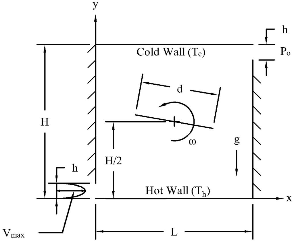
Figure 1. Schematic diagram of the computational domain along with boundary conditions
