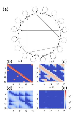
Figure 2. Response in multidimensional linear systems. Panel (a) schematically shows an example of interactions scheme for a model of the form (4). Each solid arrow represents a linear interaction coefficient 0.25, each dashed arrow stands for an auto-interaction term 0.5. The response matrix  $R_t$  is represented in panels (b)-(e) for different values of t, according to the color scheme in panel (e). Here b = 1, and correlations have been obtained by averaging over  $10^6$  trajectories.
