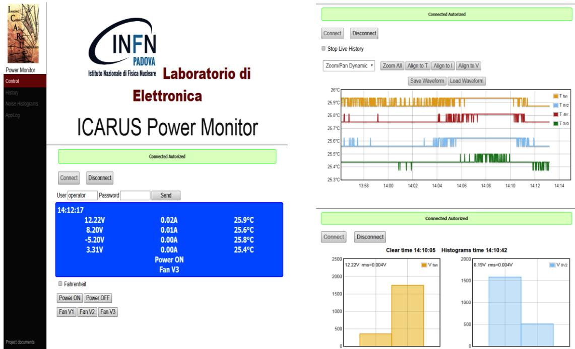
**Figure 7.** Screenshots showing the Web interface of ICARUS LVPS module. Initial page with the menu (left) and some monitors of the measured temperatures and distributions of the 12V and 8.2 V supply voltage (right).
