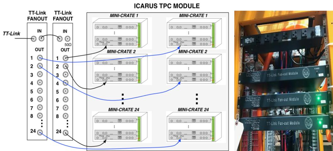
**Figure 18.** Layout of the TT-Link distribution with delay equalization (left) and the corresponding two switched on fan-out (green light on) modules on top of the rack serving one ICARUS TPC module (right).
