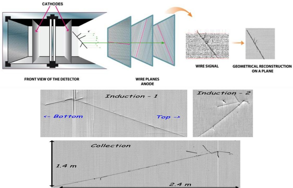
**Figure 1.** Sketch of the detector layout showing the LAr-TPC working mechanism (top). An upward-going atmospheric muon neutrino event ( $E_{\text{DEP}} \sim 1.7 \text{ GeV}$ ) collected by ICARUS-T600 at LNGS as measured in the three - Induction-1, Induction-2 and Collection - views is shown (bottom).
