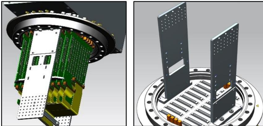
**Figure 12.** Rendering of the flange fully equipped with the DBBs held in place (left) and of the internal view of the flange with the side support of the DBB cage (right).
