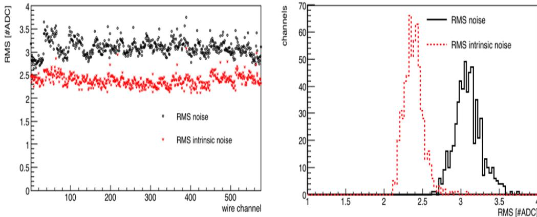
**Figure 20.** The measured RMS noise in ADC counts for the 576 channels in a mini-crate as determined by averaging over 100 events (left) and the corresponding overall 576 channels distribution (right). In each board, the first 32 channels refer to Induction-2 wires and the second 32 to the Collection wires. Black points (solid line) refer to the measured values, while the red ones (dashed line) to the intrinsic noise after the coherent component removal.
