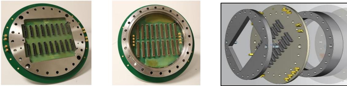
**Figure 8.** From left to right: external and internal side of the signal feed-through flange and the schematic of its basic structure. Components are glued together with a special process and vacuum/over-pressure tested by Criotec company (Turin, Italy).
