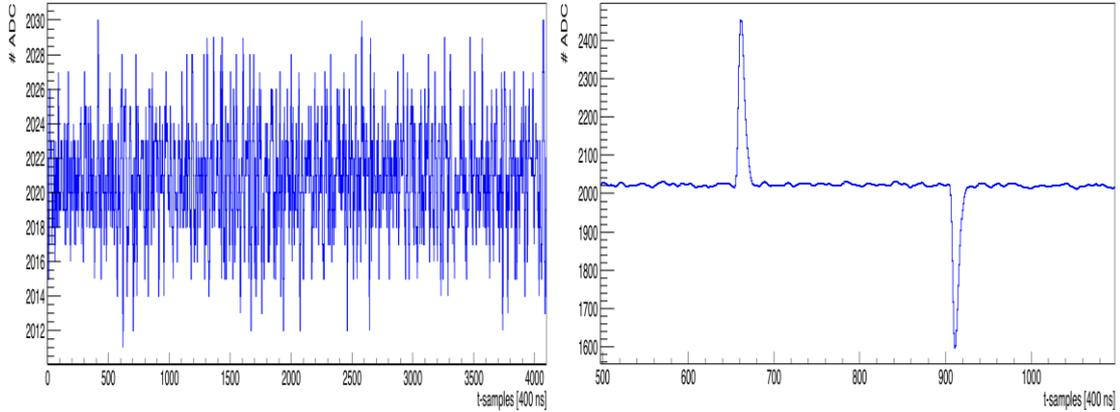
**Figure 19.** Typical baseline noise, RMS = 3.1 ADC counts without LAr in the TPC, (left, 1 ADC count corresponds to  $\sim 550$  electrons with the present 12 bit ADC) and shape of the injected test pulse as detected on one Collection wire (right).
