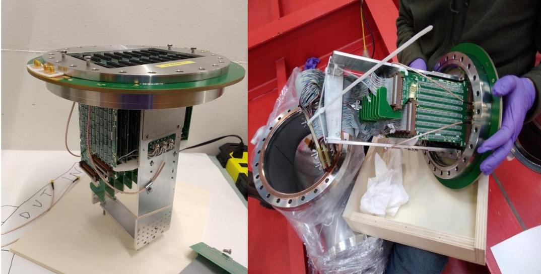
**Figure 15.** An assembled feed-through with nine DBB and the biasing cables (left). Installation of a feed-through flange on the top cross of a chimney (right). The bundle of the 18 flat signal cables and the two brown coaxial biasing cables are visible.
