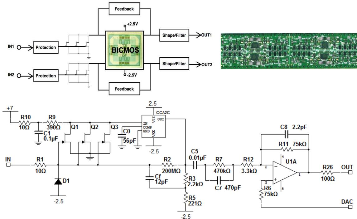
**Figure 2.** Block diagram of the front-end amplifier (top left) and PCB ( $81 \times 20 \text{ mm}^2$ ) housing 8 amplifiers with a symmetrical layout (top right). Front-end schematic (bottom). The high number of elements inside the BiCMOS prevents showing a detailed schematic here.
