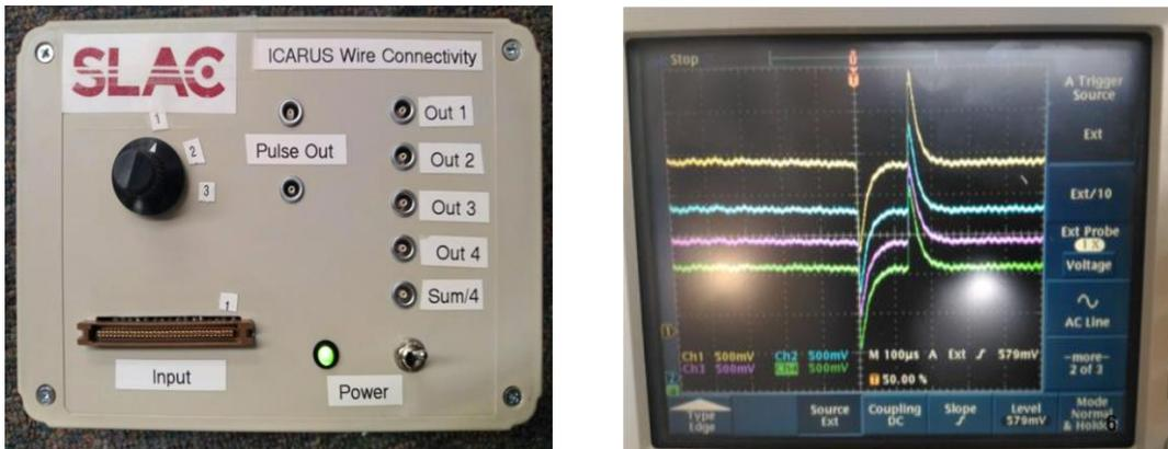
**Figure 16.** Custom-designed test box (left). Induced signals displayed on the oscilloscope (right).
