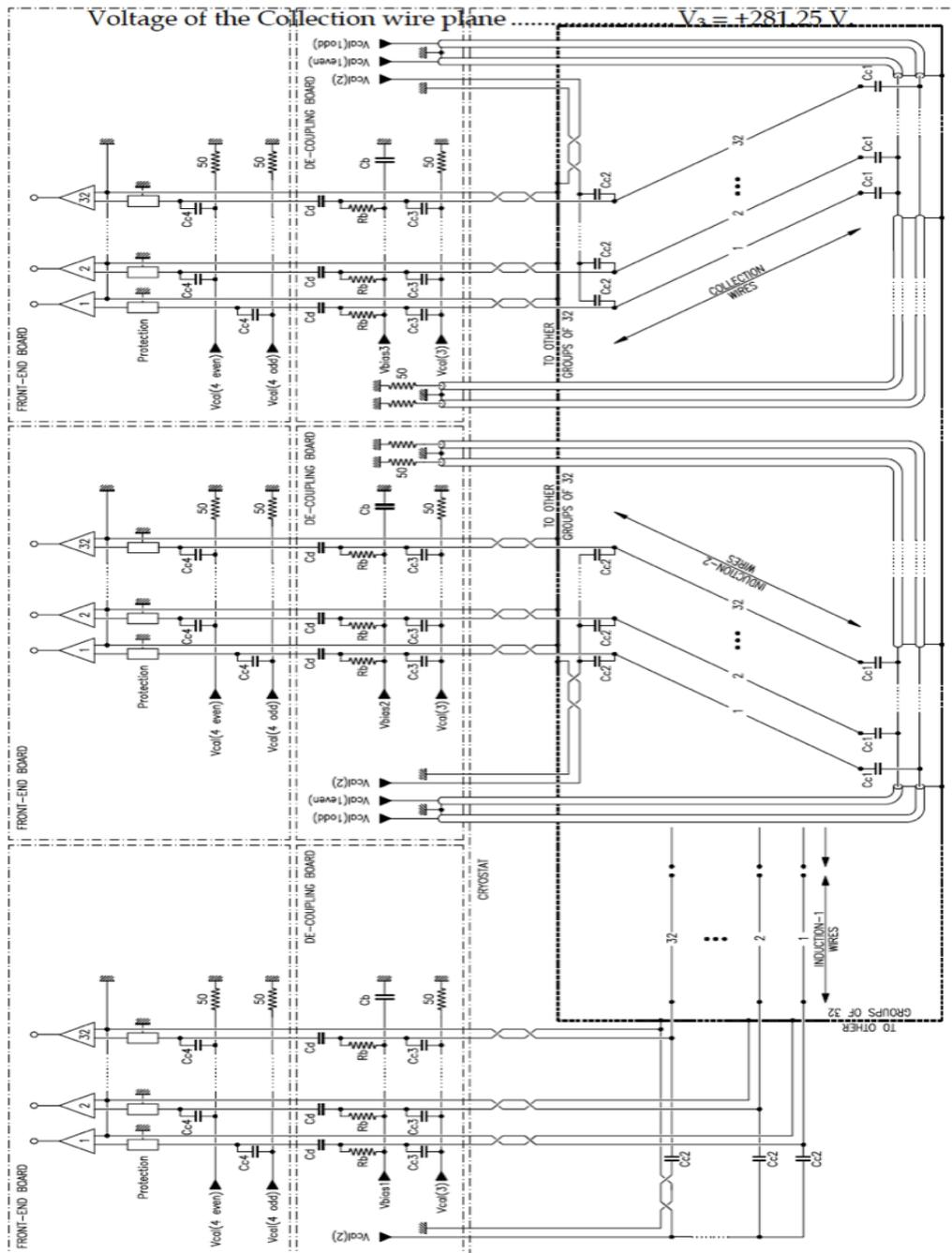
**Figure 13.** Read-out, high voltage decoupling and calibration scheme. All GND symbols are intended to be detector ground.
