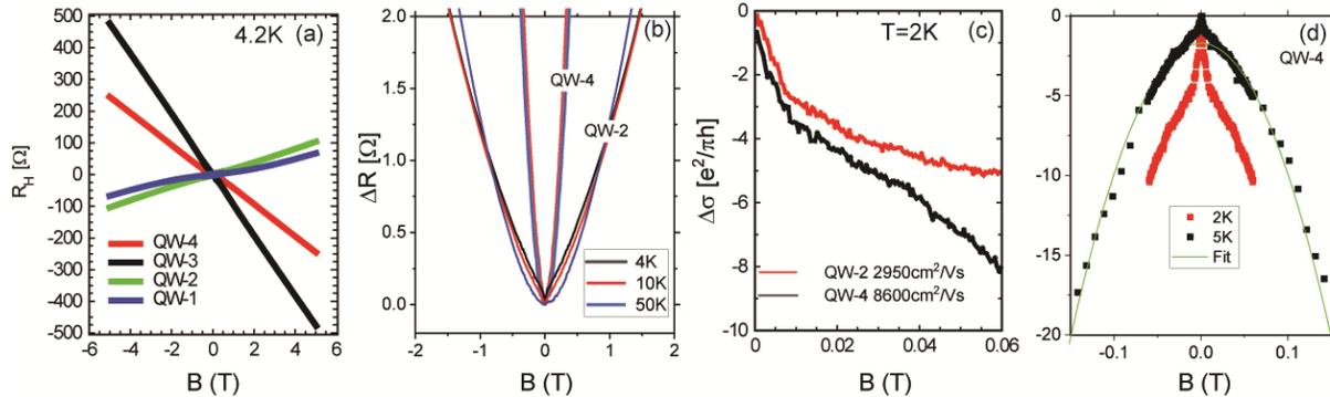
**FIG 2.** (a) Hall resistance of four QW with different Bi doping density. (b) Change in resistance versus magnetic field measured in QW-2 and QW-4 at different temperatures. (c) Magnetoconductance at low field showing weak antilocalization effect in QW-2 and QW-4 at 2K. (d) Magnetoconductance for QW-4 showing a coexisting cusp and parabolic field dependence. A curve fit is shown in green and yields a parabolic contribution equal to  $820 \pm 30e^2/(\pi\hbar T^2)B^2$ .
