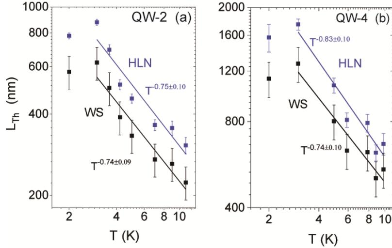
**FIG 5.** Coherence length  $L_{Th}$  as a function of temperature obtained from each model for QW-2 (a) and QW-4 (b) by fitting up to  $0.06T$ . The uncertainty on  $L_{Th}$  in the WS model is dominated by the uncertainty on the diffusion constant discussed in appendix B.
