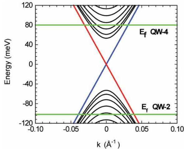
**FIG 6.** Band structure computed using the k.p formalism detailed in Appendix B and the band alignment shown in Fig. 1(a). QW subbands are shown in black and the topological interface states are shown in red and blue. The Fermi level position of QW-2 and QW-4 is shown in green. The bands are offset compared to the model parameters to have the midgap lie at zero energy. These energy bands are 4-fold valley degenerate in TCIs.
