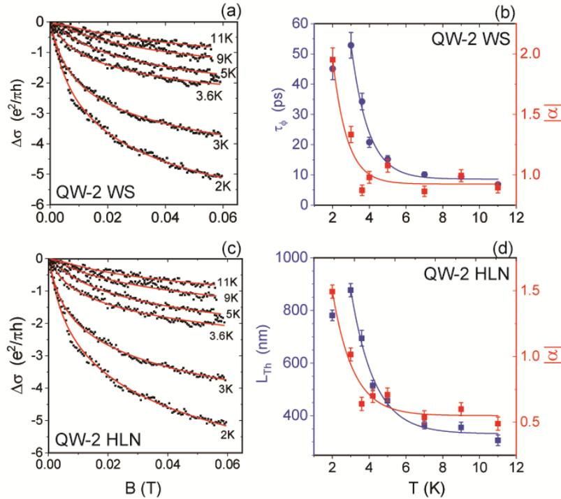
**FIG 3.** WAL analysis for QW-2. (a) WAL data at small field  $<0.06T$  ( $\approx 0.5B_{tr}$ ) from 2K to 10K. The solid red lines are the fitting curves obtained by the WS model and the points represent experimental data. (b) Fit parameters obtained from WS fitting. (c) Same as (a) with the fitting curve obtained by the HLN model. (d) Fit parameters obtained from HLN.  $\beta$  is fixed at 0 for both WS and HLN. The lines in (b) and (d) are a guide for the eye.
