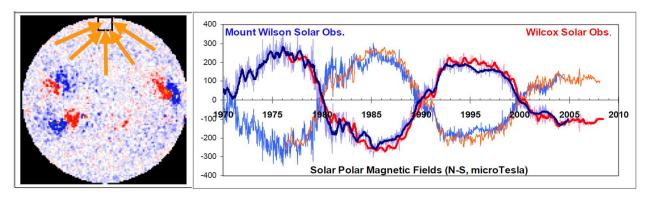
**Figure 3.** (Left) Scattering of light into the polar aperture. (Right) Time variation of the solar magnetic axial dipole moment (expressed as the difference (N-S) between the polar fields in the North (N) and in the South (S)). Also plotted is the difference between S and N (S-N). MWO data are shown with bluish colors. WSO data are shown with reddish colors. Heavy lines show 12-month running mean values of the N-S difference. Adapted from Svalgaard & Schatten (2008).
