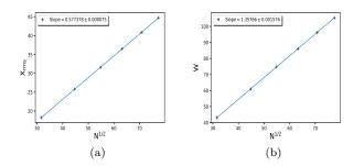
FIG. 4: Plots of the (a)  $x_{\rm rms}$  versus  $N^{1/2}$  and (b) Full width at half maximum W versus  $N^{1/2}$  for RW with random steps  $R_n$  in descending order are shown and find straight lines with slopes equal to 0.57737 and 1.3576 respectively.
