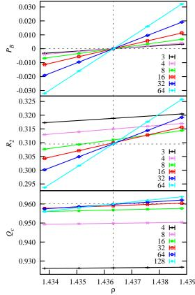
FIG. 10: Plots of  $P_{\rm B}$ ,  $R_2$  and Q versus  $\rho$  for different system sizes L for the continuum percolation model. Values of L are given in the legend. Vertical dashed line shows the threshold  $\rho_c = 1.436\,325\,05(10)$ , and horizontal dashed lines indicate the universal values of these quantities at criticality. The error bars of the data are smaller than the size of the data points. The solid lines connecting data points are added for clarity.
