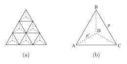
FIG. 2: (a) The star-triangle transformation on the triangular lattice; (b) One individual star-triangle with the bond probabilities p and  $p^*$ .
