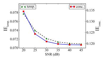
Fig. 6. Dependency of IEs for the reconstructed distributions of  $H_2O$  concentration and temperature at different SNRs.
