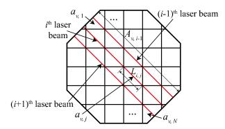
Fig. 1. Geometric description of CST measurements in the discretised RoI.
