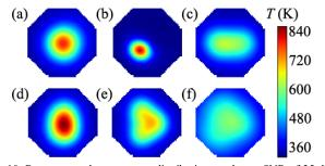
Fig. 10. Reconstructed temperature distributions under an SNR of 35 dB for the corresponding phantoms shown in Fig. 8.
