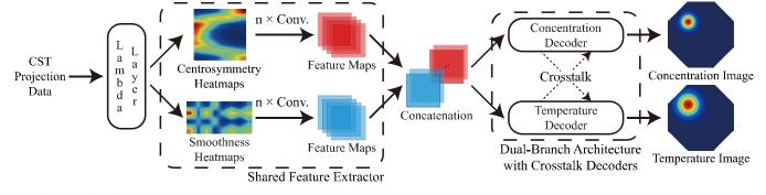
Fig. 3. The overall architecture of CSTNet.
