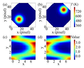
Fig. 2. Illustration of *a priori* information of centrosymmetry in CST. (a) and (b) are two centrosymmetric temperature images; (c) and (d) are the heatmaps containing  $A_{\nu_1}$  and  $A_{\nu_2}$  obtained from the temperature images in (a) and (b), respectively.
