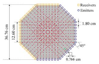
Fig. 4. Optical layout of the 32-beam CST sensor.
