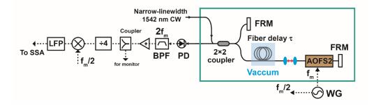
**Fig. S2** Experimental setup for fiber noise measurement. FRM, faraday rotating mirror; AOFS, acoustic optical frequency shifter; BPF, bandpass filter; LPF, lowpass filter; PD, photodetector; PI: proportional-integral servo; PID, proportional-integral-differential servo; WG, waveform generator.
