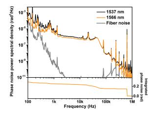
Fig. S3. In-loop residual phase noise PSD of 1537-nm and 1566-nm comb modes
