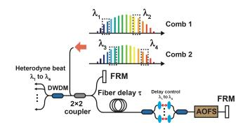
Fig. S5. Design of relatively narrow-linewidth dual-comb system. FRM, faraday rotating mirror; DWDM, dense wavelength division multiplexer; AOFS, acoustic optical frequency shifter.
