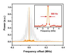
Fig. 4. Linewidth measurement of  $f_{\text{beat}}$  before (grey curve) and after (orange curve) phase-locking. Inset: the linewidth is estimated to be 580 Hz from Gaussian fit.
