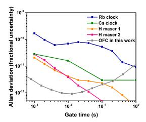
**Fig. S4.** Allan deviation of Rb clock (blue curve), hydrogen maser 1 (orange curve), hydrogen maser 2 (pink curve), Cs clock (green curve) and *f*<sub>beat</sub> (grey curve).
