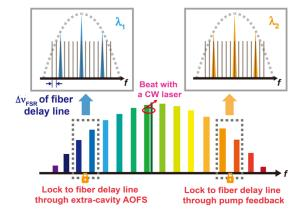
Fig. 1. Scheme of optical frequency comb reference to a fiber delay line
