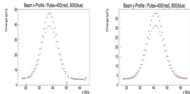
Fig. 6: x/y beam transverse profiles of single pulses measured by the 2D Ionization chamber prototype, after more than 100 cm in air.
