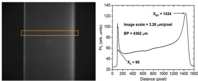
Fig. 9: (Left) Bragg curve fluorescence image stored in a LiF crystal irradiated at 1.8 m from the exit of SCDTL-4. (Right) PL intensity profile versus depth in LiF in the selected yellow marked rectangular region.
