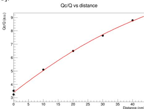
Fig. 5: Dependence of the coefficient of proportionality ( $Q_c/Q$ ) between the IC\_B and the corresponding Faraday Cup collected charges, as a function of the distance of the IC\_B from the beam exit window. The curve is a fit of the measured points; details in the text.
