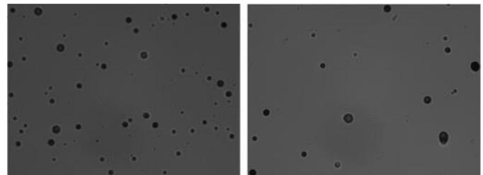
Fig. 8: Photographs (magnification 40X) of the etched tracks in a CR39 detector irradiated with 1 Gy, showing a typical field on the rear side (left panel) and front side (right panel) of the CR-39.
