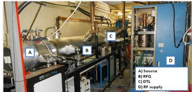
Fig. 2: the PL7 Injector. A) Source, B) the radiofrequency quadrupole, C) the drift tube linac, D) the radiofrequency supply.
