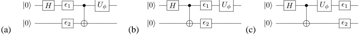
Figure SC1: Noisy Circuit with noise channels  $\epsilon_1$  and  $\epsilon_2$ . (a) Noise before the CNOT gate. (b) Noise after the CNOT gate. (c) Noise after the phase rotation gate.
