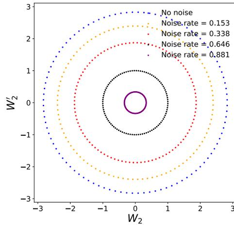
Fig SC3: Phase trajectories for the uncorrelated amplitude damping channels located after the CNOT/phase gate.
