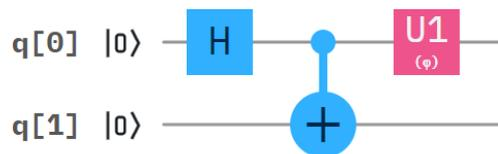
Figure SB: Operating on  $q[0] \otimes q[1]$  with the Hadamard gate and the CNOT gate.
