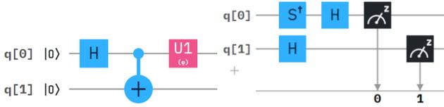
Fig. 1: (a) The quantum circuit for a 2-qubit GHZ-like state,  $|\text{GHZ}_2\rangle = \frac{1}{\sqrt{2}}(|00\rangle + e^{i\varphi}|11\rangle)$ .  $H$  represents the Hadamard gate,  $UI(\varphi)$  is a gate that rotates a quantum state about the  $z$  axis to impart phase  $\varphi$ , and  $CNOT$  gate entangles the two qubits. (b) The quantum circuit of  $YX$  measurement for the 2-qubit pair.
