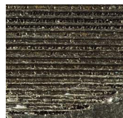
Zoomed view of grooves with mechanically smoothed craters on indicated fragment of LMT.
