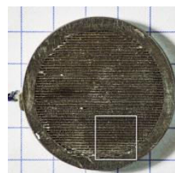
Back Side of Target Prototype with laser engraving and mechanically smoothed craters in grooves (LMT)
