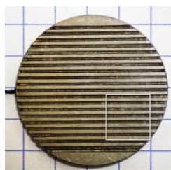
Back side of mechanically milled target prototype (MMT).
