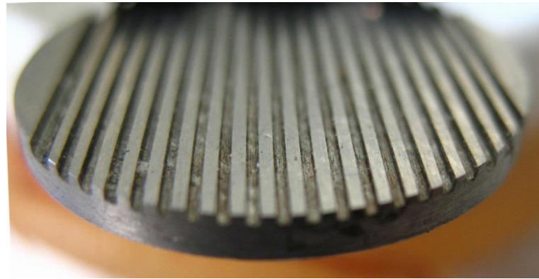
Smooth grooves on back side of mechanically milled target prototype (MMT).
