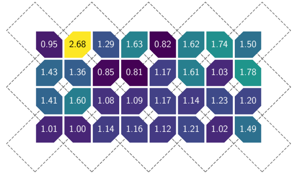
FIG. S11. Two-qubit gate percent Pauli error obtained by cross-entropy benchmarking (XEB), where non-conflicting subsets of two-qubit gates are applied simultaneously. These values were measured against the standard \sqrt{\text{iSWAP}}^\dagger without the parasitic controlled phases. The two-qubit gates are calibrated using our routine calibration process without Floquet calibration, see Section V in the Supplementary information in [39].
