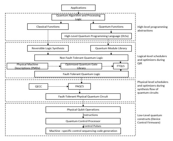
Fig. 5: Quantum module implementation (series of compiler transformations and optimizations to translate high-level quantum program into specific hardware instructions)
