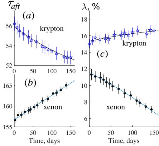
**Figure 3.** The variation of electrons drift time from the cathode to the anode ( $\tau_{aft}$ ) and the ratio of the amplitudes of the afterpulse to the primary pulse ( $\lambda$ ) for long-term measurements at filling of the CPC with krypton and xenon performed in the same conditions.
