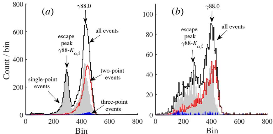
**Figure 2.** Pulse height spectrum from the external  $^{109}\text{Cd}$  source located in the middle of the CPC length. *a* - the CPC is filled pure Xe with total pressure of 5.0 bar; no quenching or accelerating gases are added. *b* - the same sample, but containing micro additions of oxygen and hydrogen sublimated from the inner surfaces of the detector walls after 4000 hours of counter operation.
