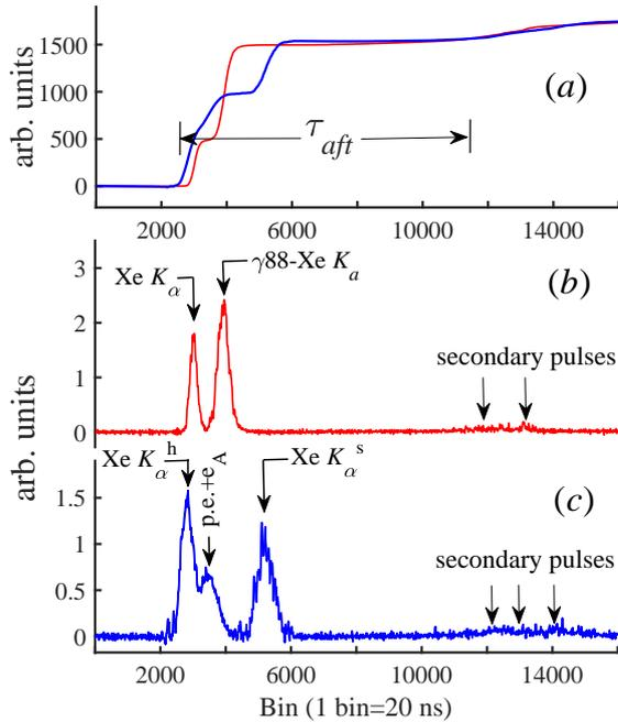
**Figure 1.** (a) - examples of charge pulses from CSA corrected for self-discharge from two- (red curve) and three-point events (blue curve). Current pulses for two- and three-point events, (b) and (c) respectively.  $\tau_{aft}$  is the duration of the electron drift from the cathode to the anode.
