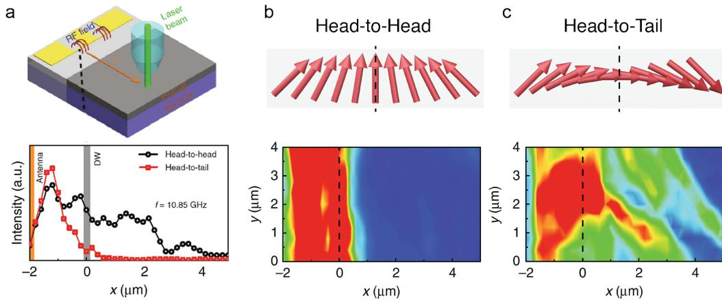
Figure 24: (a) Spin waves propagating across domain walls detected by  $\mu$ BLS in a CoFeB/BaTiO<sub>3</sub> bilayer system. Spin waves are excited by a stripline antenna at 10.85 GHz and travel across different types of domain walls resulting in different amplitudes. Two dimensional spin-wave intensity maps are presented in (b) Head-to-Head and (c) Head-to-Tail domain walls. Reproduced from Ref. [163].
