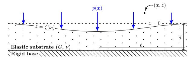
Figure 1: A cross-section sketch of the general setup considered in this paper: the surface (at z = 0) of a threedimensional elastic block adhered to a rigid base (at z = -d), with aspect ratio  $\epsilon := d/\ell \ll 1$ , is displaced by a pressure field  $p(\mathbf{x})$ . The position of the deformed surface is  $z = \zeta(\mathbf{x})$ .
