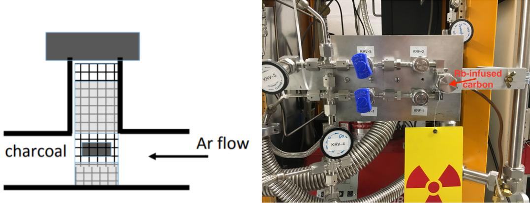
**Figure 6.** **Left:** Diagram of carbon location within the VCR tee. A structure of thin steel mesh and fine quartz wool holds the carbon in place within the tee. **Right:**  $^{83\text{m}}\text{Kr}$  source attached to the CENNS-10 gas-handling system in operation mode focused on the VCR tee holding the carbon and surrounding parts. The VCR tee is the section in the center on the right side of the source.
