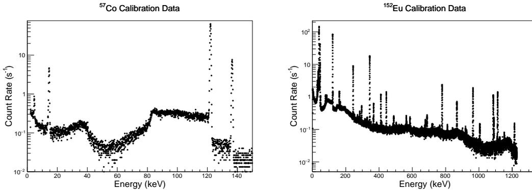
**Figure 3.** **Left:** Data from the  $^{57}\text{Co}$  calibration used for the activity measurement. A run length of 300 s was taken with a source with an activity of 27.71 kBq at the time of the measurement. **Right:** Data from the  $^{152}\text{Eu}$  calibration for the activity measurement. A run length of 900 s was taken with a source with an activity of 193 kBq on May 15, 2010
