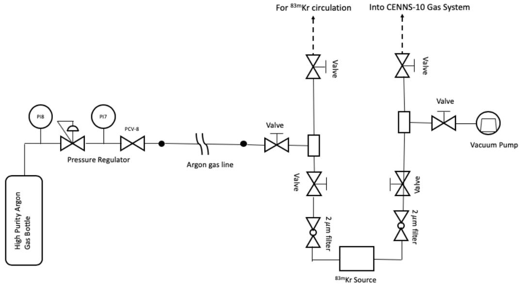
**Figure 5.** CENNS-10  $^{83\text{m}}\text{Kr}$  source plumbing diagram. The source attaches directly to the CENNS-10 gas-handling system. If necessary, the source can be bypassed to flow GAR directly into the detector. The  $^{83\text{m}}\text{Kr}$  source is contained in a 1/2 in. VCR cap and tee holding the  $^{83}\text{Rb}$ -infused carbon.
