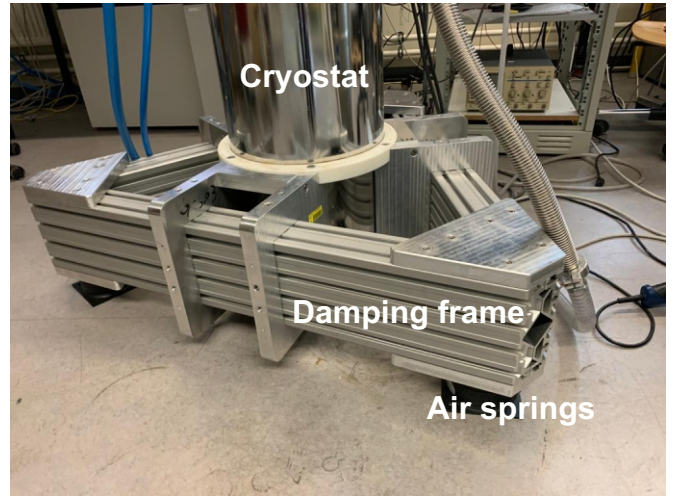
Figure 8. Damping stage for the cryostat equipped with air springs to compensate ground vibrations.
