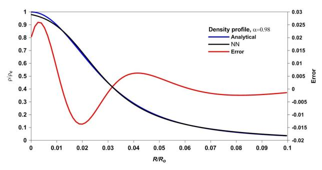
Figure 7: The fractional density profiles obtained in the validation phase. The maximum relative error is 2.5%.
