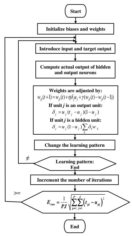
Fig 2. Flowchart of an off-line back-propagation training algorithm
