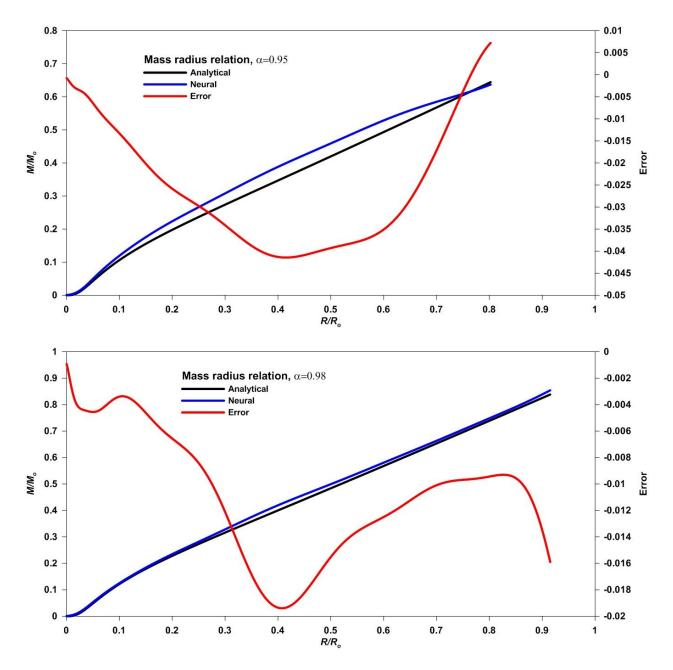
Figure 9: The fractional mass-radius relations obtained in the validation phase. The maximum relative error is 4%.
