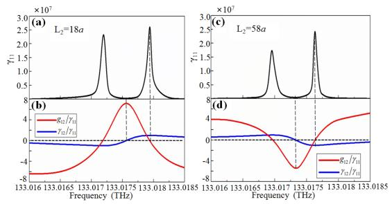
FIG. 2. Spontaneous decay rates of single QE  $\gamma_{11}$  (black lines) for two cases (a)  $L_1=L_3=20.5a$ ,  $L_2=18a$  and (c)  $L_1=L_3=15a$ ,  $L_2=58a$ . (b) and (d) represent the coherent (red lines) and incoherent (blue lines) coupling parameters for these two cases.
