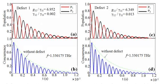
FIG. 5. Populations (a) and entanglement concurrence (b) of two QEs as a function of time for the case of the first defect with f=133.0175 THz,  $g_{12} / \gamma_{11} = 6.952$  and  $\gamma_{12} / \gamma_{11} = 0.002$ . The curves in (c) and (d) have the same meaning with (a) and (b) for the case of the second defect with f=133.0175 THz,  $g_{12} / \gamma_{11} = 6.349$  and  $\gamma_{12} / \gamma_{11} = 0.013$ .
