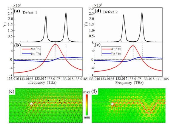
FIG. 3. Spontaneous decay rates of single QE  $\gamma_{II}$  (black lines) for two defects, (a) defect 1 and (d) defect 2; (b) and (e) represent the coherent (red lines) and incoherent (blue lines) parameters for the cases of two defects; (c) and (f) are simulated unidirectional propagation of the state along the interface for the two defects respectively. The stars represent chiral light sources near the interface.
