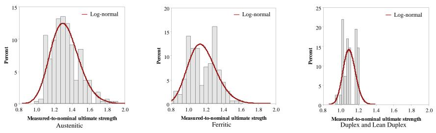
Figure 5. Histograms of ultimate strength  $f_u$  for different cold-formed stainless steel types.
