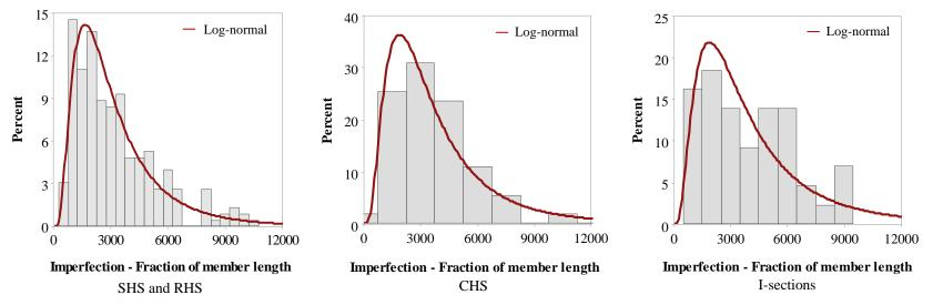
Figure 8. Histograms of member imperfection amplitudes for different stainless steel section types.
