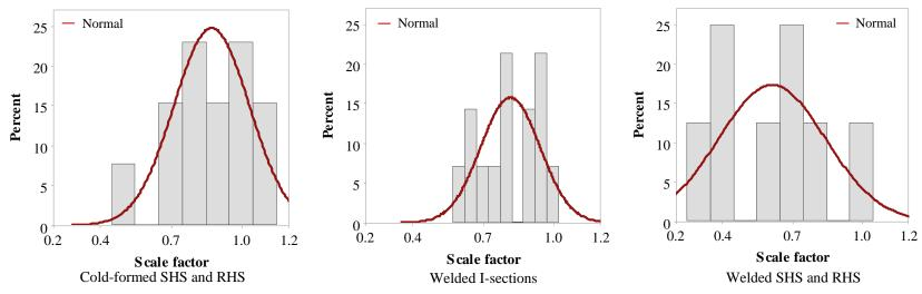
Figure 9. Histograms of residual stress magnitude scale factors for different stainless steel section types.
