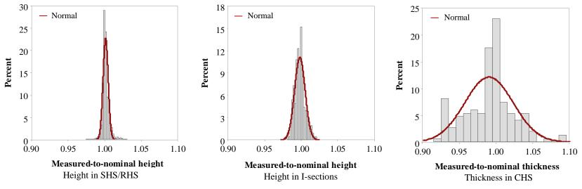
Figure 2. Histograms of cross-section dimensions for different stainless steel section types.
