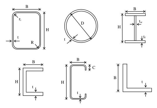
Figure 1. Variables on cross-section properties for different section types.
