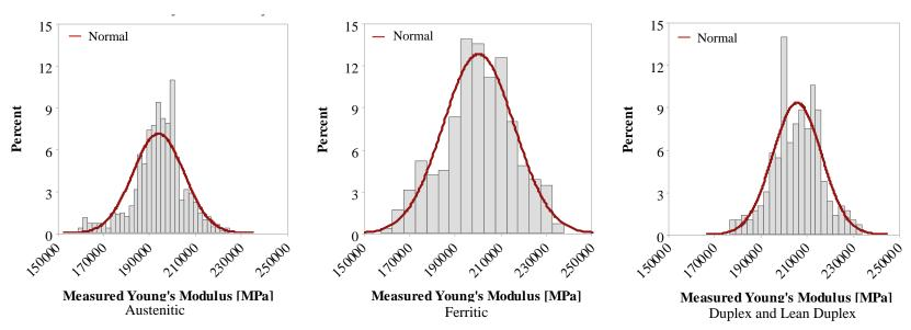
Figure 3. Histograms of Young's modulus E for different stainless steel types.
