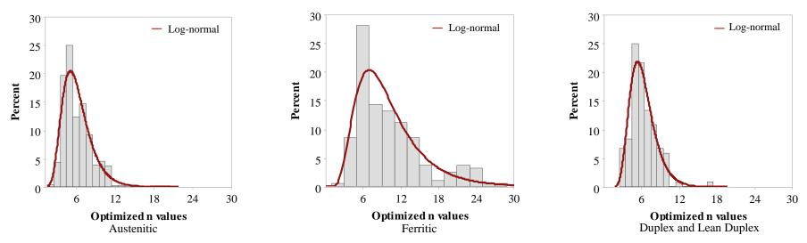
Figure 6. Histograms of strain hardening exponent n for different cold-formed stainless steel types.
