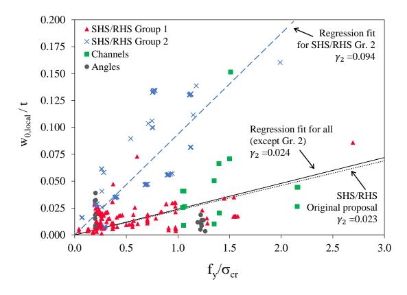
Figure 7. Assessment of predictive models for local imperfection amplitude in stainless steel cold-formed sections.
