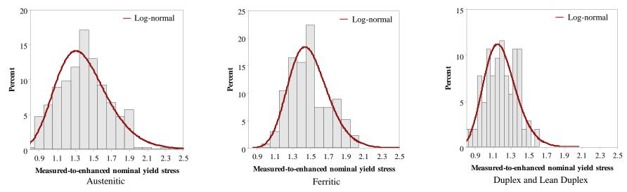
Figure 4. Histograms of yield stress f<sub>v</sub> for different cold-formed stainless steel types.
