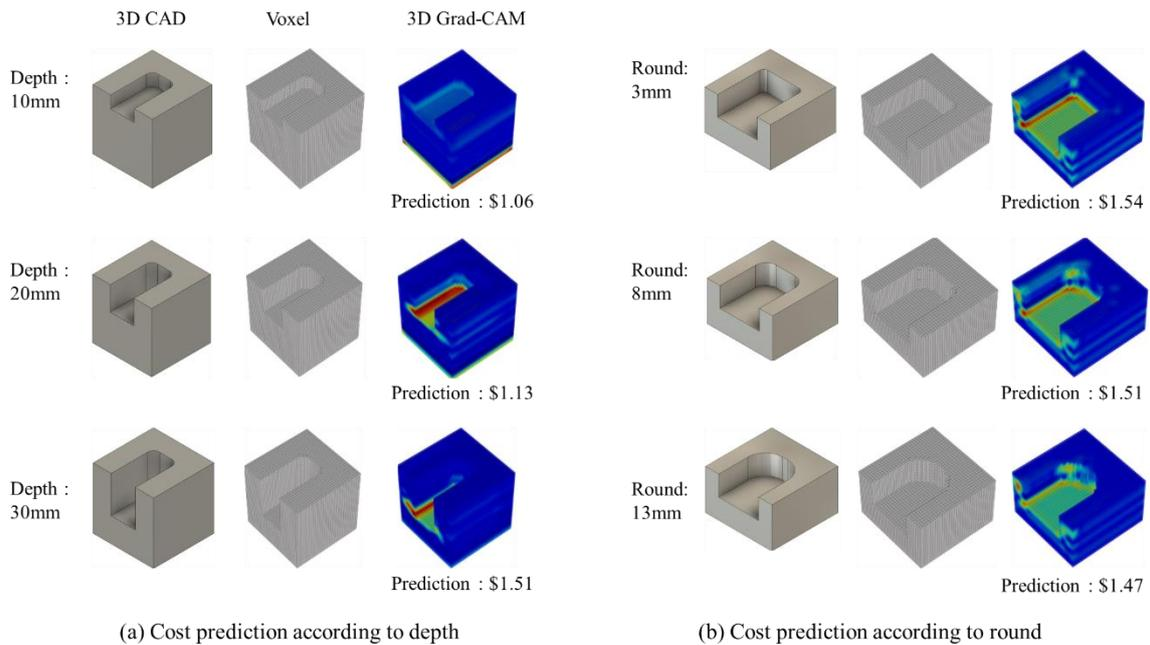
Fig. 17. Recognition of difficulty of machining processing
