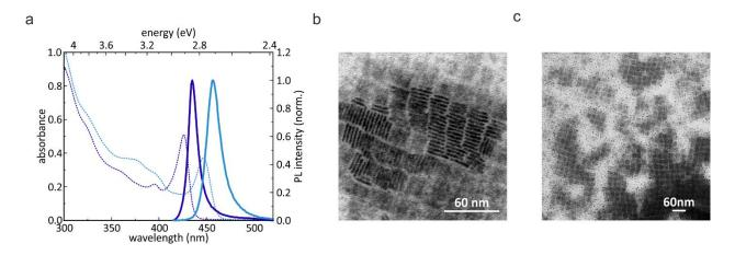
Figure 1. Thickness-controlled halide perovskite nanoplatelets (NPls). a) Absorption (dashed lines) and PL (solid lines) spectra of 2 ML (purple) and 3 ML (blue) NPls. b,c) TEM images of 2 ML NPls from which a thickness of  $1.3 \pm 0.2$  nm and side lengths of  $19 \pm 1$  nm are determined.
