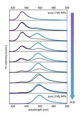
**Figure 2.** Energy transfer between NPIs in thin films. PL spectra (colored lines) of mixed 2 ML and 3 ML NPI thin films obtained via drop-casting and ranging from pure 2 ML (top) to pure 3 ML NPIs (bottom). Shown in black are the calculated PL spectra obtained by adding the pure 2 ML and
